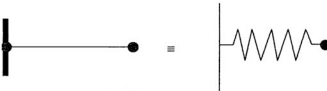
Fig. 4.61. Equivalent spring system
