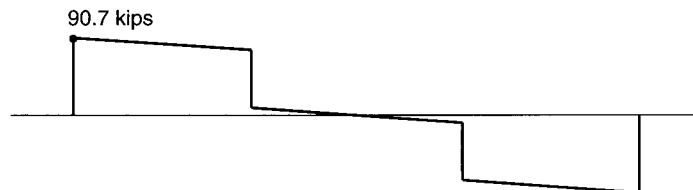
(b) Shear design envelope, V_u/\phi , for loading in part (a).
