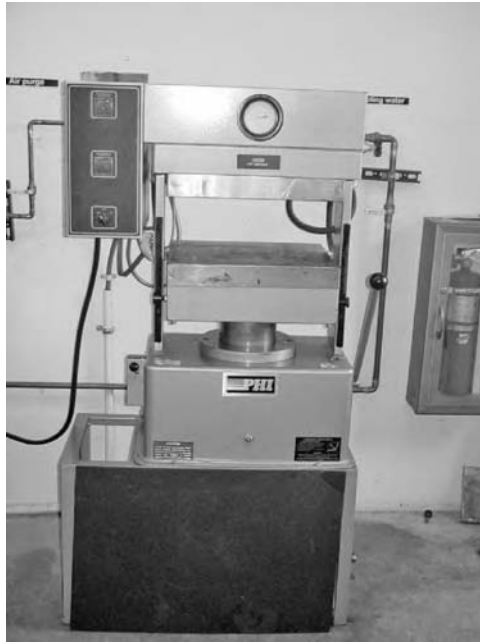
FIGURE 3.12 Compression molding equipment. (Courtesy of CFC, West Virginia University.)
