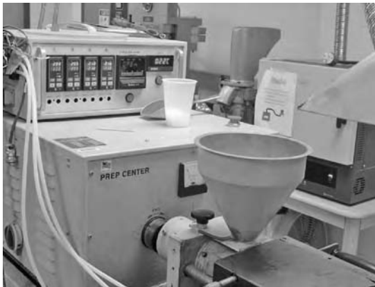
FIGURE 3.15 Temperature control for four different heat zones in the extrusion equipment used by the CFC, West Virginia University.
