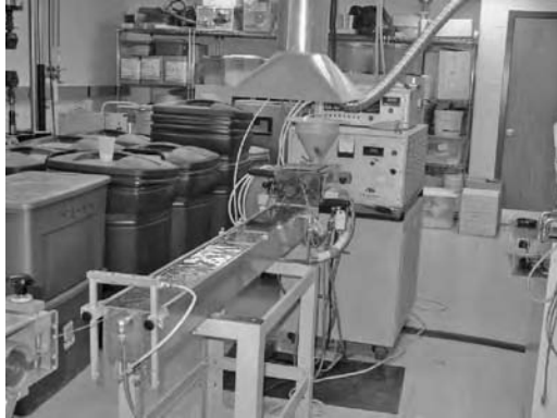
FIGURE 3.14 Extrusion equipment used by the CFC, West Virginia University.
