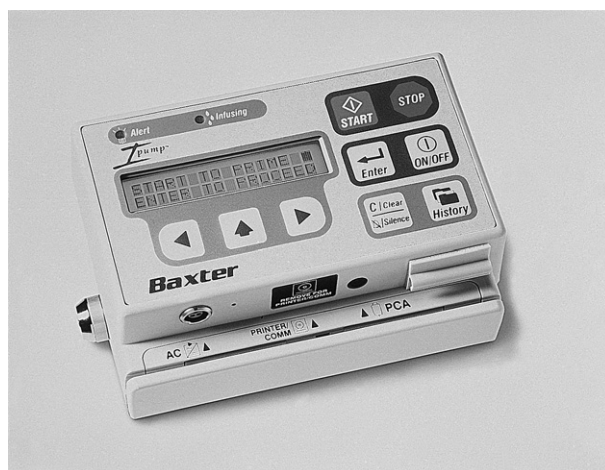
FIGURE 72.2 PCA pump. Not shown is the patient call button, which is attached to the pump and allows the patient to request medications. (Reproduced with permission from Baxter Healthcare, Round Lake, Illinois.)
