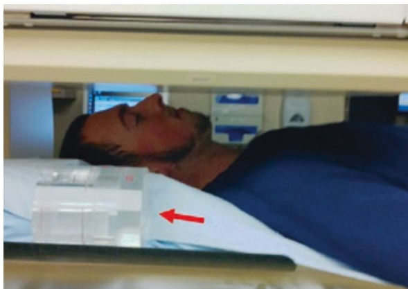
Fig. 4.9 Gamma camera with parallel-hole collimator for imaging and uptake measurements. Neck phantom with standard activity in the field of view ( arrow )
