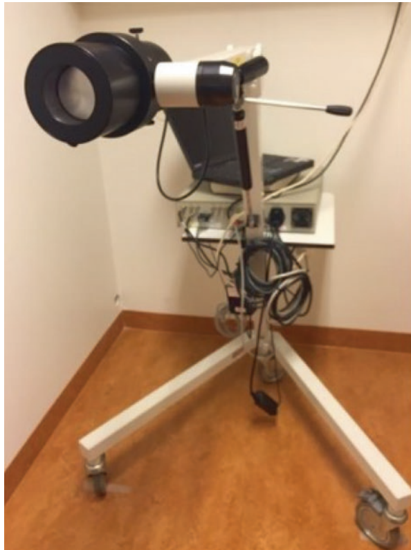
Fig. 4.8 Thyroid probe for uptake measurements
