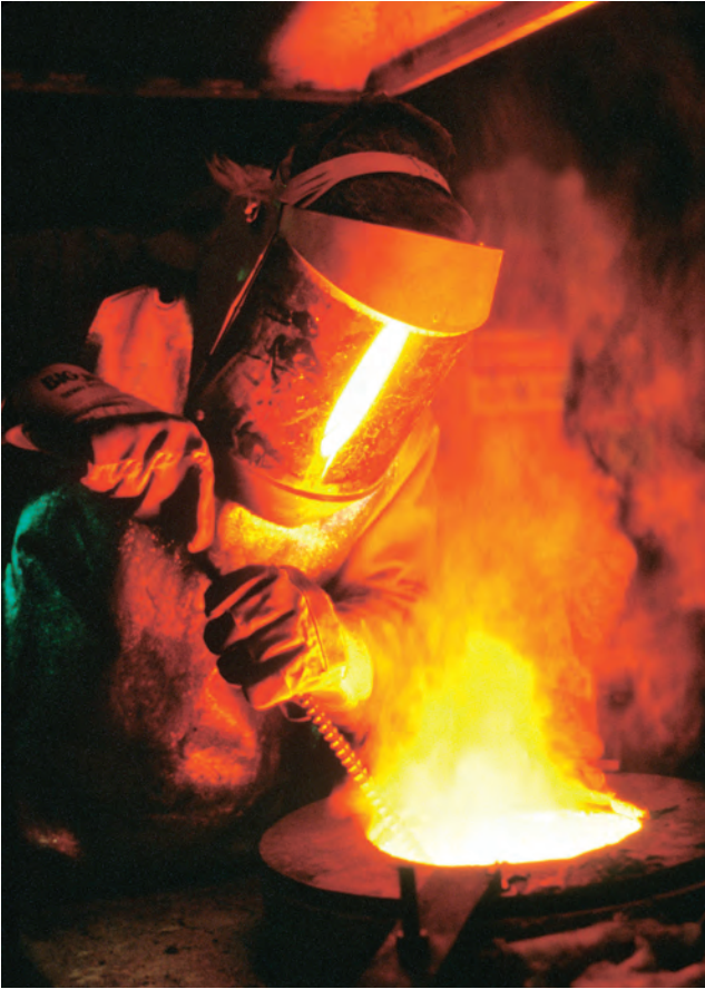
Figure 15.11 Metal furnace – source of infrared heat
