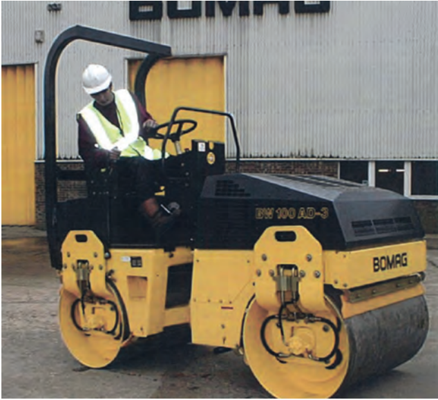
Figure 11.36 (a) Ground consolidating rider-mounted vibrating roller
