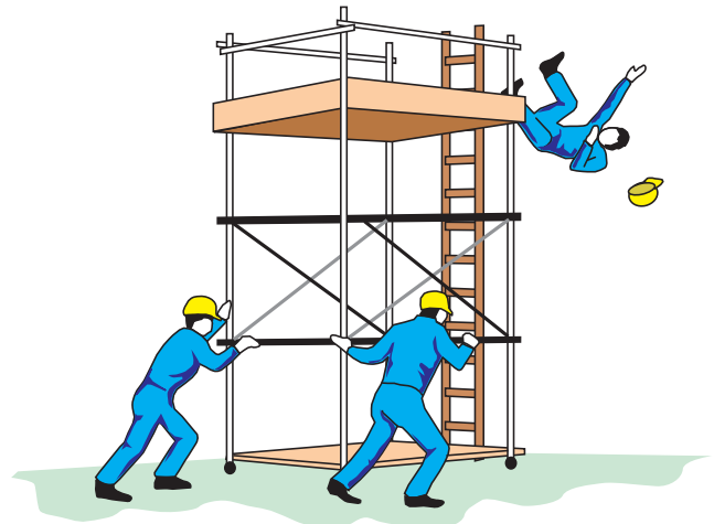
Figure 8.14 Falling from a height – tower scaffold with inadequate handrail (too low) and no middle rail. Access ladder should be internal and it should never be moved with people on the scaffold
