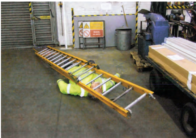
Figure 5.6 Accident at work – reconstruction of a ladder accident showing where the deceased person was found under the ladder which had toppled over while he was attempting to adjust the height of the extending ladder
