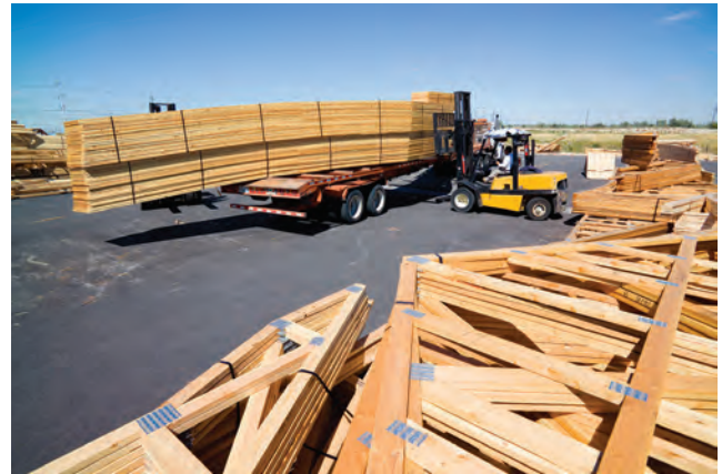
Figure 9.15 Fork-lift truck loading timber trusses onto a trailer. Loading vehicle correctly and evenly is most important for road stability en route
