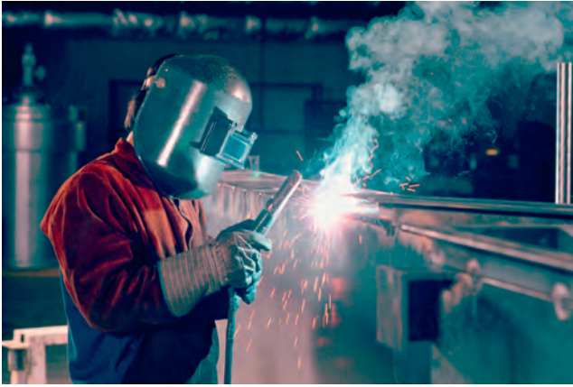
Figure 22.2 High level of fumes from welding
