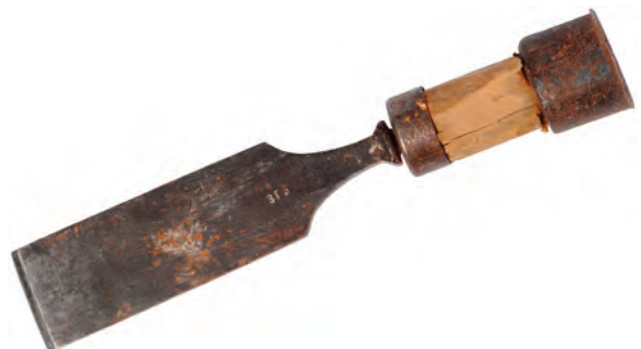
Figure 11.8 (a) broken and dangerous wood chisel handle
