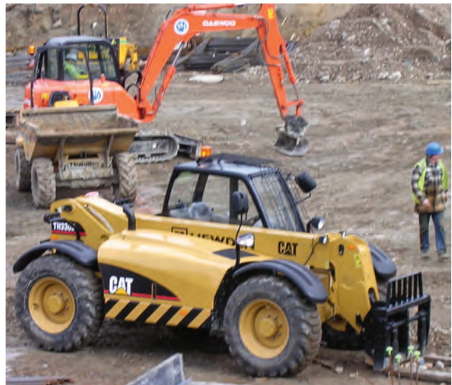
Figure 9.2 Various construction plant with driver protection
