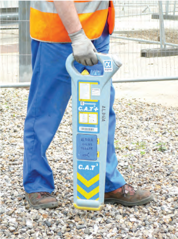
Figure 12.10 Checking for underground cables with a cable detector
