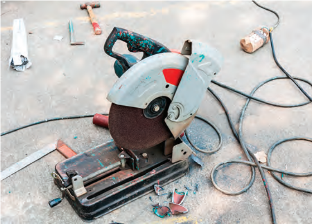
Figure 12.4 Electrical faults through overloading or damaged cables cause a large number of fires on construction sites (see Chapter 13)
