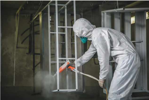
Figure 14.2 Paint spraying – risk of sensitising particularly if isocyanate based paint used and inadequate local exhaust ventilation
