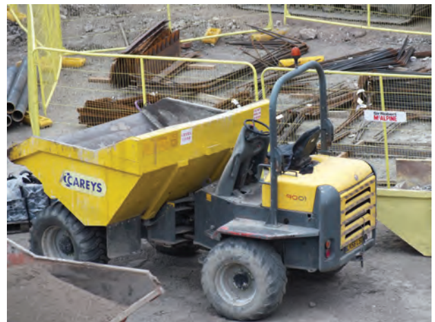
Figure 9.4 Dumper truck with rollover protection (ROP)
