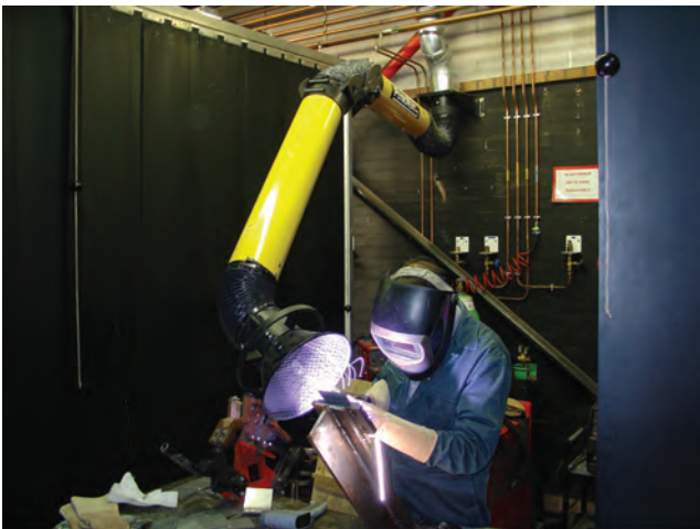
Figure 14.12 (a) Common elements of a simple LEV system; (b) welding with an adjustable LEV system to remove dust and fumes
