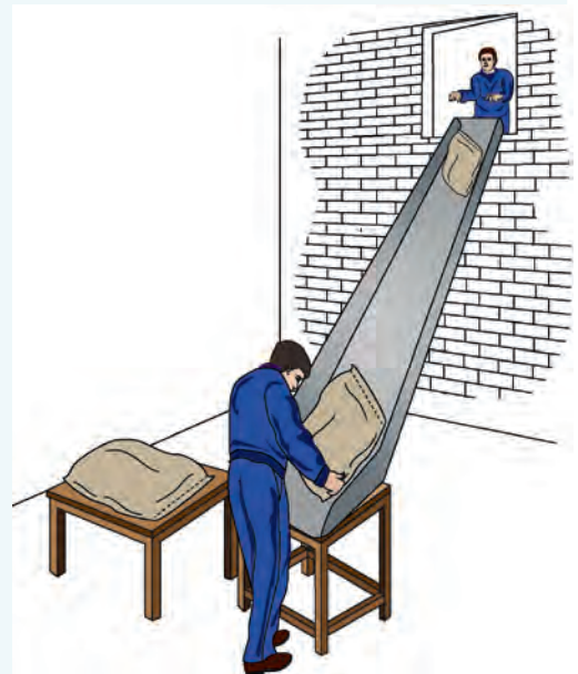
A chute being used to transfer sacks from a high to low level
