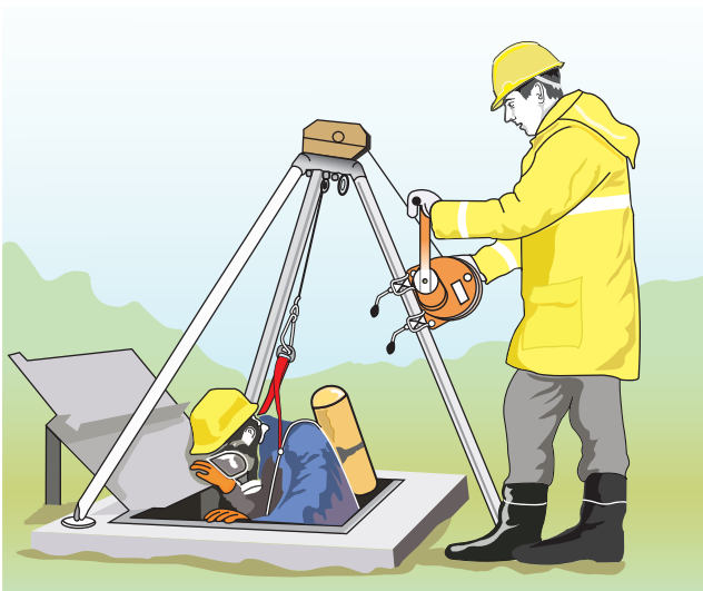
Figure 4.26 Entering a confined space with breathing apparatus, rescue tripod and rescue watcher
