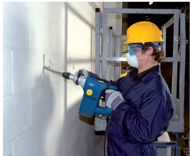
Figure 11.11 Electric drill with percussive hammer action to drill holes in masonry
