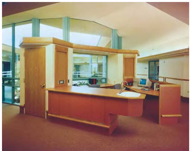
5.7.6 A nurses' station, triangular in configuration, with charting counters and sink for handwashing. Two storage supply closets flank an open workspace. A large picture window affords visual surveillance of the courtyard/atrium. Note the full height glass along the corridor
