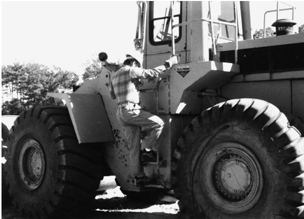
FIGURE 7.60 Construction worker mounting heavy equipment using three points of contact
