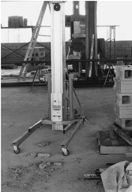
FIGURE 11.23 An example of a material lift
