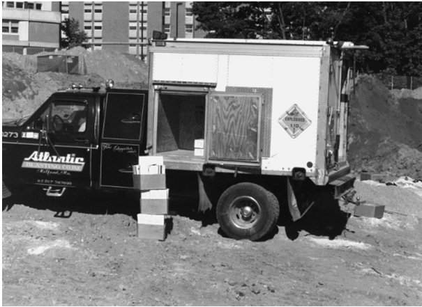
FIGURE 7.41 Typical vehicle used by those transporting explosives
