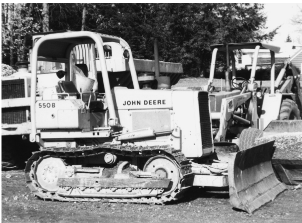
FIGURE 8.29 Dozer with rollover protection and overhead protection
