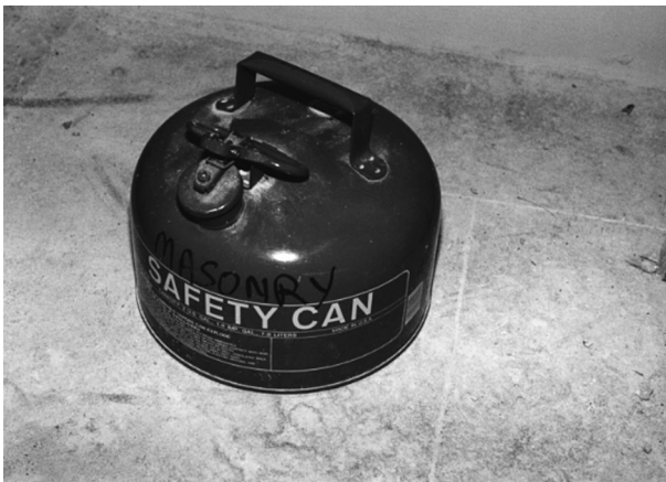
FIGURE 9.26 Gasoline and flammables should be stored in approved cans
