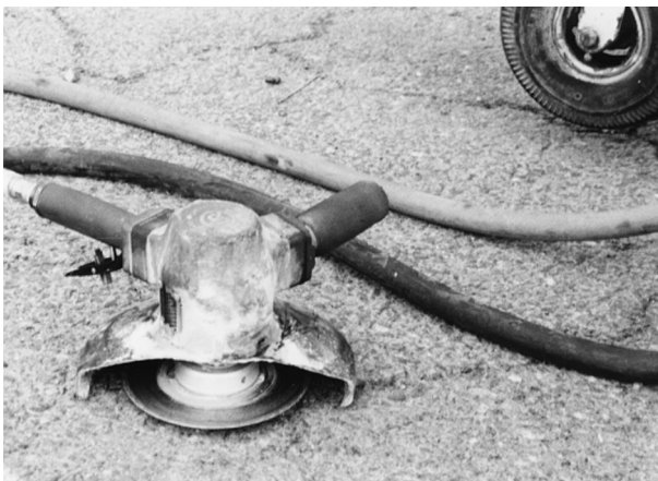
FIGURE 8.13 Example of pneumatic driven grinder
