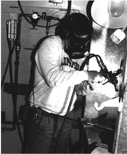
FIGURE 9.30 Worker “personal” exposure monitoring and “area” monitoring
