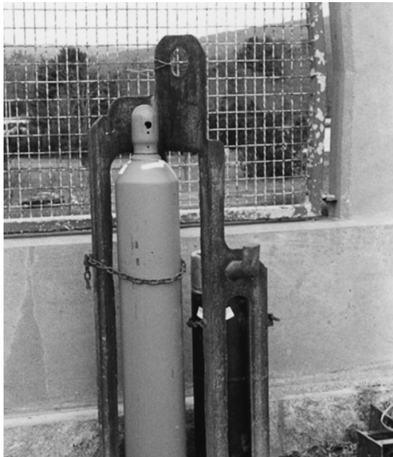
FIGURE 7.8 Cradle for lifting compressed gas cylinders
