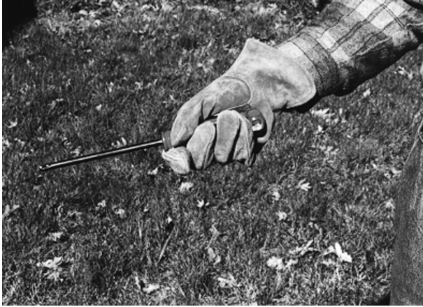
FIGURE 11.21 The use of gloves requires longer handles since grip strength is also reduced by gloves
