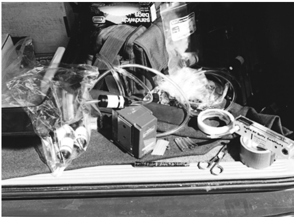
FIGURE 9.29 Monitoring apparatus for field asbestos survey
