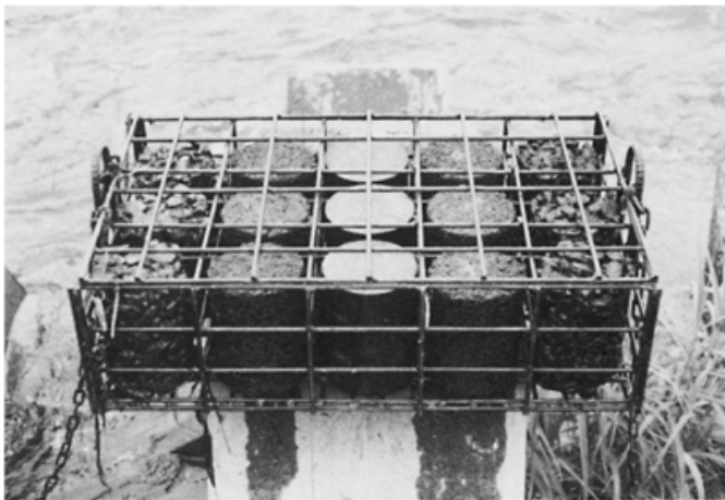
Photo. 1. Underwater exposure test specimens
