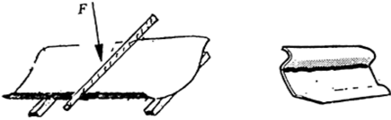
Figure 6. Sketch of the testing arrangement to BS 550 and the direction of crack propagation
