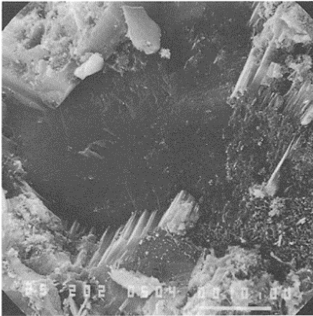
Figure 4(a) Calcium hydroxide on the surface of aggregate particles in an ordinary mortar
