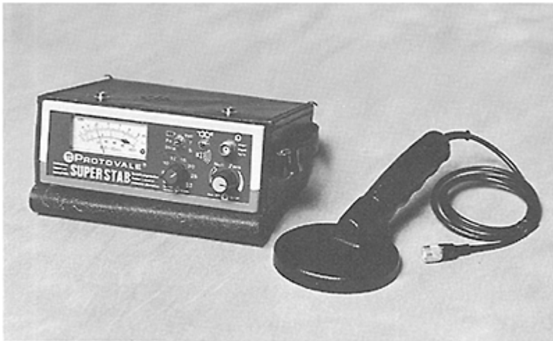
Figure 2 Photograph of “SuperStab”: the first version of a stainless-steel cover meter
