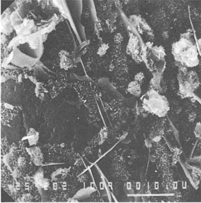
Figure 4(b) Calcium hydroxide in a mortar containing 0.100M self-cure admixture.
