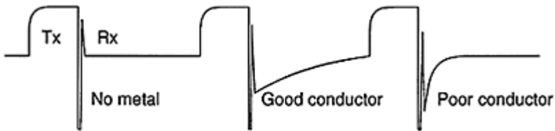
Figure 1 Coil pulse waveforms in the absence and presence of conducting metal
