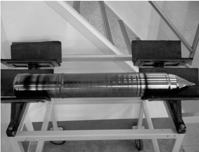
Figure 3.2. A purified silicon ingot used in photovoltaic solar power technology.
