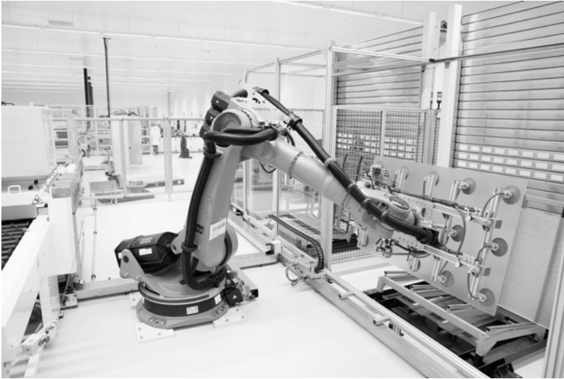
Figure 3.8. Robotic PV module assembly.
