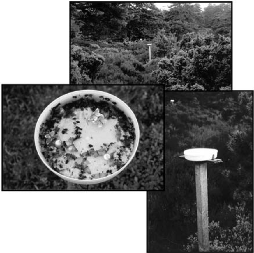
Fig. 6.4 Simple water trap. Insects are attracted to settle on the bright surface and become trapped in the water.
