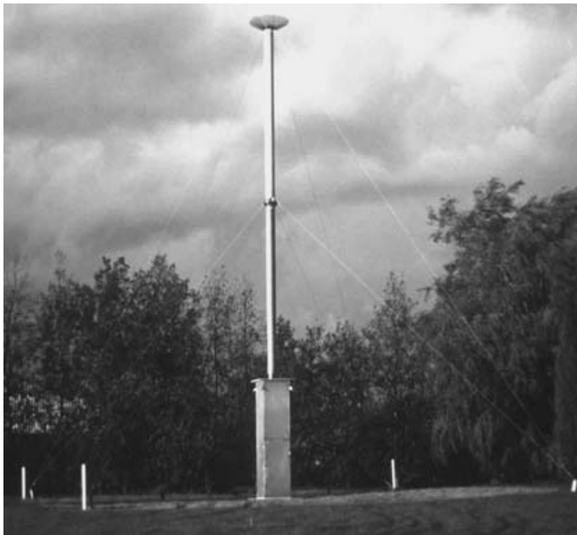
Fig. 6.2 Rothamsted Insect Survey standard design suction trap. These are used to provide warning of increasing aphid numbers in spring and early summer. Picture courtesy of Ian Woiwod, Rothamsted Experimental Station.
