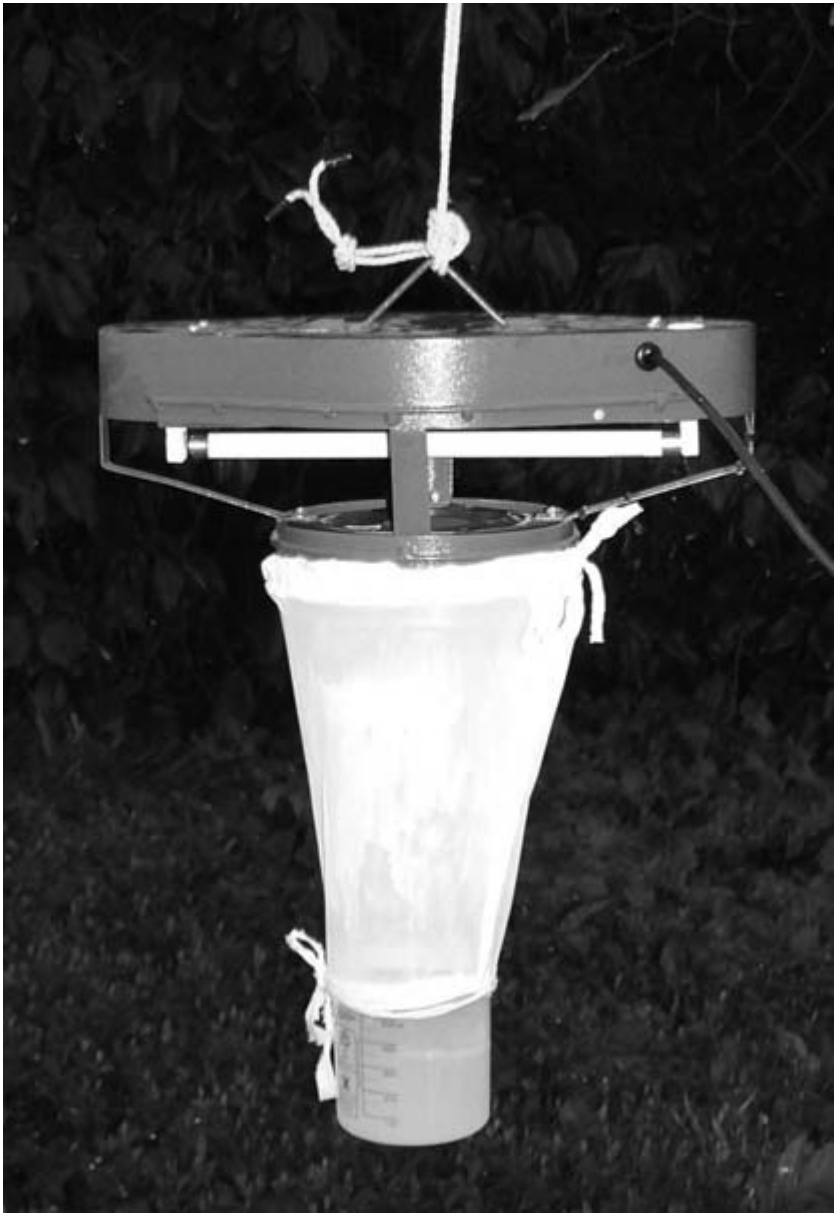
Fig. 6.3 Onderstepoort Veterinary Institute design combined light and suction trap. Small insects are attracted by the light and then sucked down into the collecting chamber.
