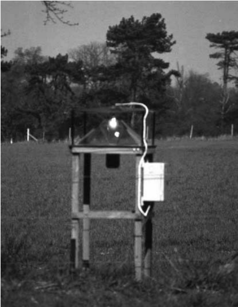
Fig. 6.1 Rothamsted Insect Survey standard design light trap. These are used in long-term monitoring of moth populations. Picture courtesy of Ian Woiwod, Rothamsted Experimental Station.
