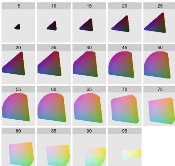
**Fig. 6.2** The shape of the HCL colour space. Hue is mapped to angle, chroma to radius and each slice shows a different luminance. The HCL space is a pretty odd shape, but you can see that colours near the centre of each slice are grey, and as you move towards the edges they become more intense. Slices for luminance 0 and 100 are omitted because they would, respectively, be a single black point and a single white point
