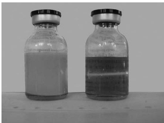
FIGURE 5 (See color insert.) Two nanosuspensions composed similarly, produced by high-pressure homogenization, conventional method (left) versus translucent nanosuspension (particle size well below 100 nm) resulting from H96 technology. The red laser beam is reflected by the tiny nanocrystals. Source : From Ref. 40.
