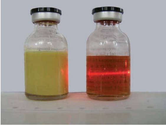
FIGURE 5.5 Two nanosuspensions composed similarly, produced by high-pressure homogenization, conventional method ( left ) versus translucent nanosuspension (particle size well below 100 nm) resulting from H96 technology. The red laser beam is reflected by the tiny nanocrystals. Source : From Ref. 40.
