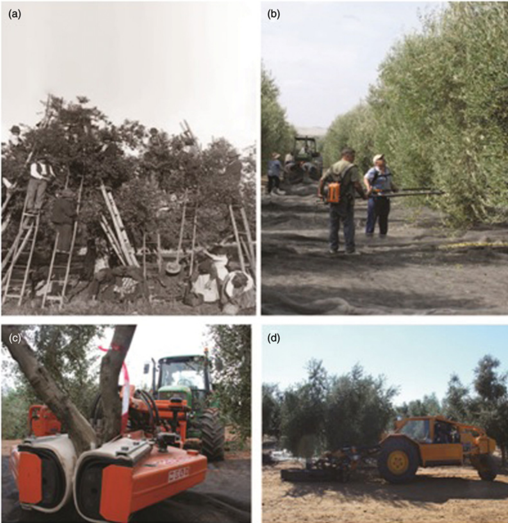
Figure 6.1 Hand olive harvesting and tools to facilitate fruit removal process: (a) hand harvest. Source: Courtesy of d’Abrunhosa family. (b) Handheld combing. (c) Trunk shaker mounted in tractor. (d) Self-propelled trunk shaker.
