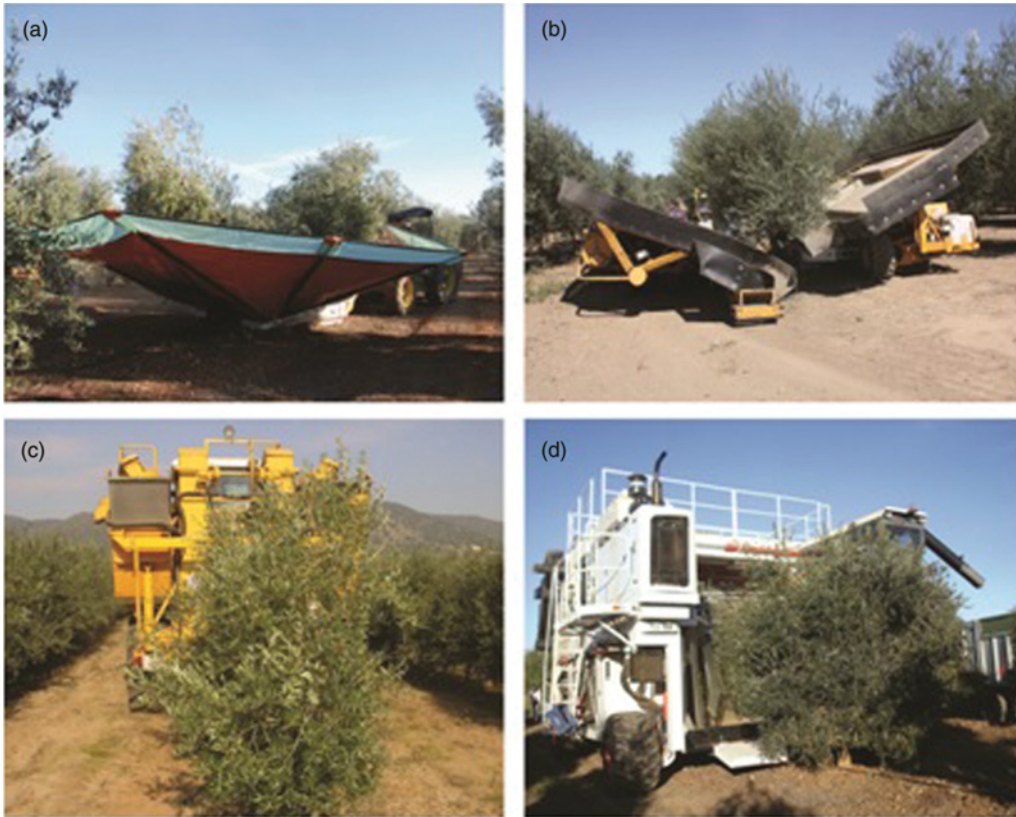
Figure 6.2 Olive harvesters: (a) trunk shaker with an inverted umbrella catch frame, (b) side-by-side trunk shaker, (c) modified vineyard straddle harvester, and (d) canopy shaker straddle harvester.
