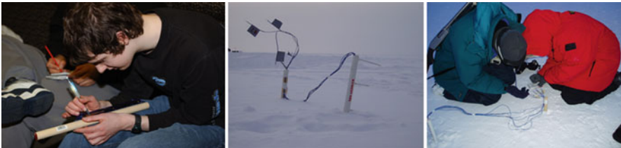
Fig. 6 Students build thermocouples in teams and then work with scientists to properly install the instruments in the snow (Photo credit: Schools on Board)
