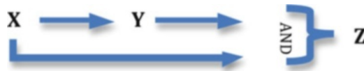
Fig. 1 The coherent feed forward loop ( FFL ) with AND gate. When X is activated, it activates Y and Z . In order to activate Z , both X and Y must be present (hence the AND logic). This simple structure has an interesting dynamical property, because it introduces a time delay between X and Z activation. This is due to the time needed for Y to accumulate before it can activate Z . Because only long enough inputs will eventually activate Z , this structure can act as a filter for signals (For more details, see Alon 2007)
