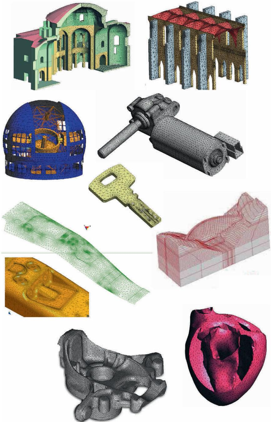
**Fig. 1.1** Discretization of different solids and structures with finite elements
