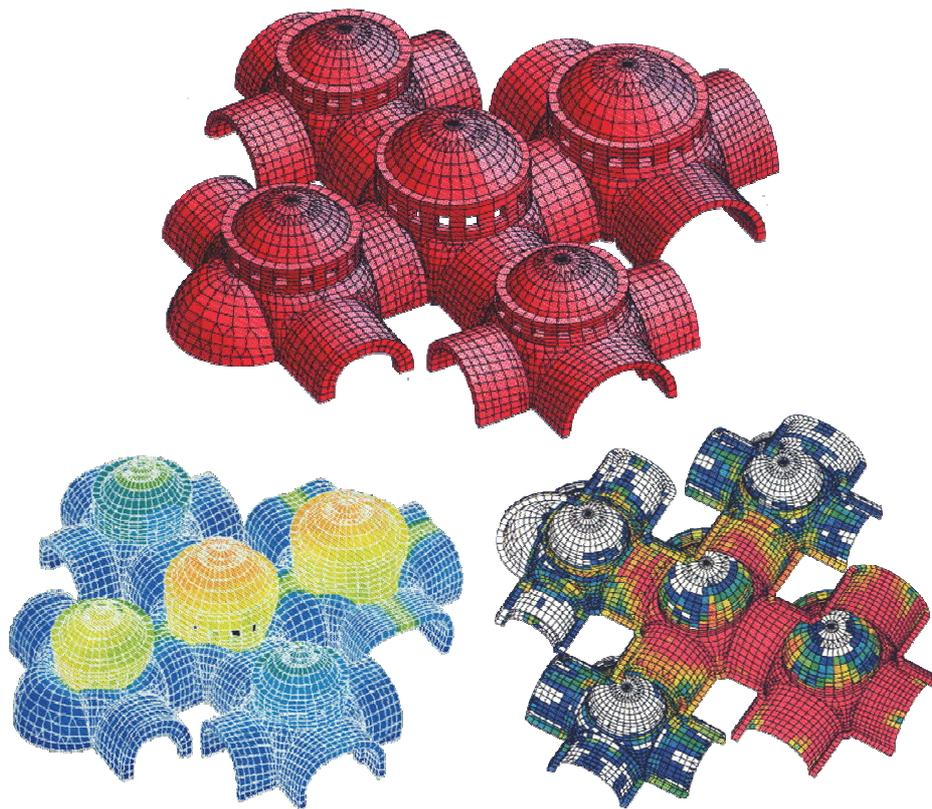
**Fig. 8.32** Analysis of Saint Mark's Basilica in Venice using 20-noded hexahedra. (a) Mesh. (b) Contours of displacement modulus under self weight. (c) Underneath view of damaged zones for an increased value of the weight [OHBO+]
