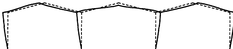
Figure B.2 Arching failure of rafters
