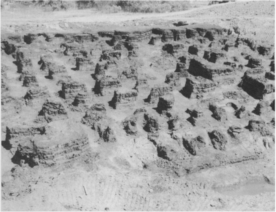
Exposed Shallow Mineworkings—"Stinking Coal" West Midlands
