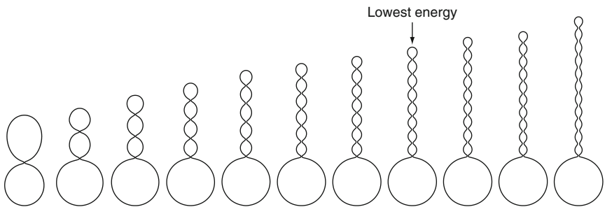
Figure 12 The shape profiles corresponding to the local minima of functional (14) for the reduced volume \nu = 0.7 , the spontaneous curvature c_0 = 12 , and without the constraint for the length. The solution with the lowest energy is the one with eight small beads.
