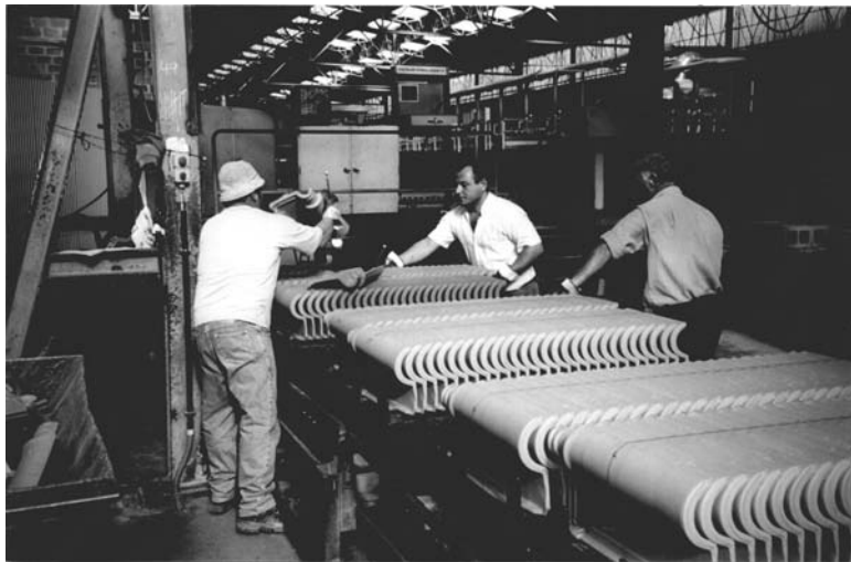
Fig. A1.7 Highly automated roof tile factory (Portugal). Quality control was undertaken best by experienced workers, following problems with mechanised systems.
