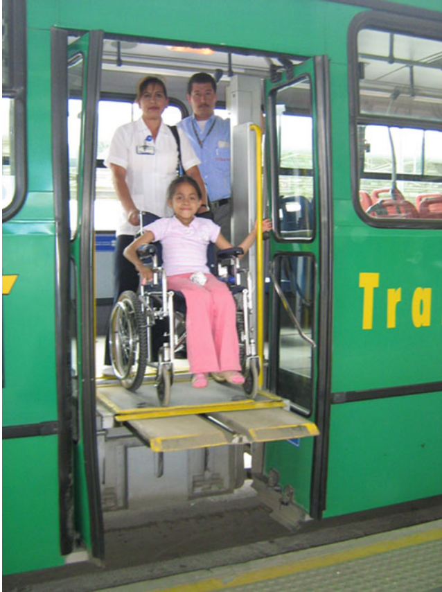
Fig. 10.8 Elevator in a feeder bus. Presentación general transmilenio (Power Point). December 2008
