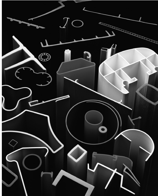
FIGURE 6–1 (See color insert.) Bending stress depends not only on the amount of cross-sectional area but also on how that area is distributed. Designers have a wide variety of shapes available, including plastic extrusions like those pictured here.
