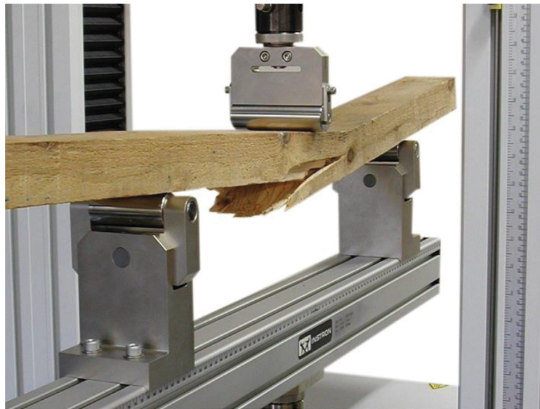
FIGURE 8-1 Wood beams are particularly susceptible to failure not due to bending stresses as calculated in the last chapter, but instead due to failure in shear. In many applications, designers must take care to analyze shear stress to avoid failures like the one shown in this test fixture.
