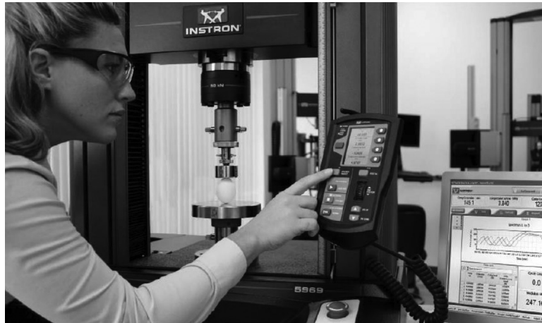
FIGURE 2–1 (See color insert.) Understanding the properties of a material is critical to achieving safe and effective designs. Test equipment, such as that shown here, is available to determine the performance of a wide variety of materials with regard to strength and deformation.
