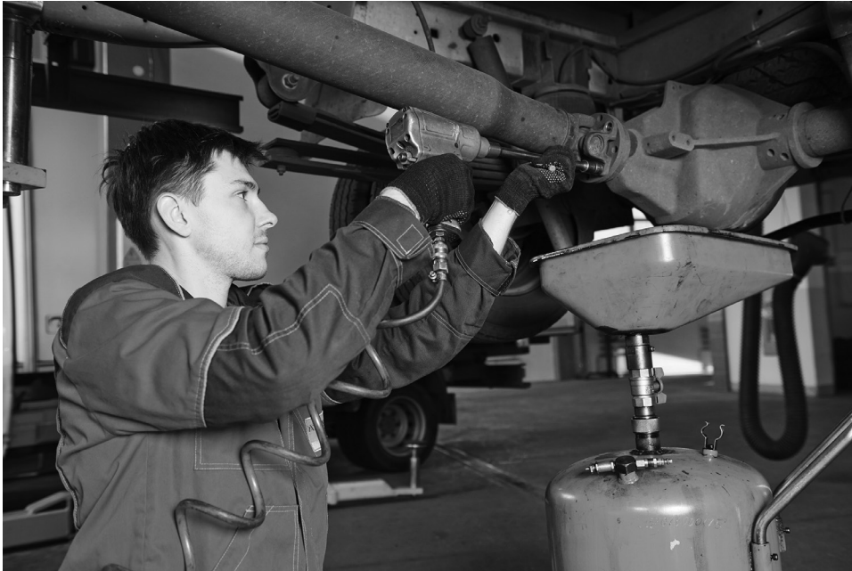
FIGURE 4-1 (See color insert.) We depend every day on elements that are loaded in torsion. In this illustration, the driveshaft over the mechanic’s head transmits torque generated by the engine to the wheels of the vehicle. Also, since the mechanic is holding a torque gun in his right hand to tighten and loosen fasteners, the relatively small shaft that he holds with his left hand is loaded in torsion as well. Designers are responsible for limiting the amount of stress and deformation in these types of components.
