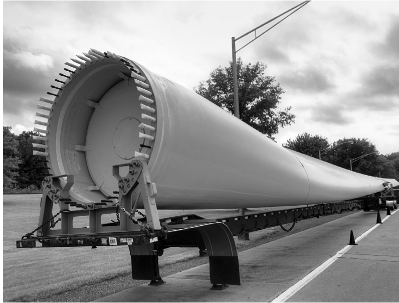
FIGURE 2–22 Large composite wind turbine blade at the installation site.
