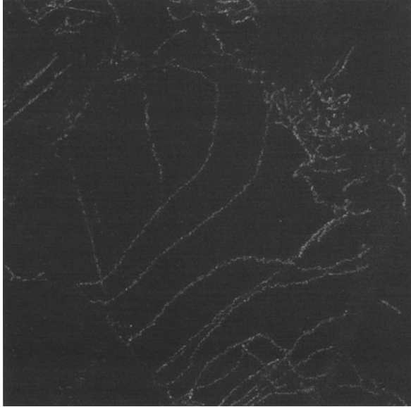
Figure 3: Dislocation structure formed on a glide plane in a large grain. The figure shows a thin slice of the grain, containing the slip planes where a dislocation pile-up has formed. The dislocations were nucleated in the grain boundary in the upper left corner, and are moving towards the lower right corner. The elastic repulsion between the dislocations keep them apart and prevent them from moving into the grain boundary, the dislocation thus form a pile-up. A few other dislocation on nearby slip planes are also seen, some of them appear to end where they move out of the slice included in the figure.
