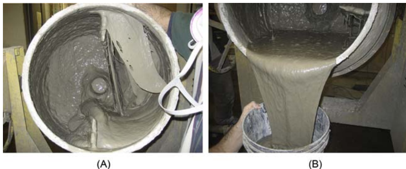
Figure 15.5 (A) Mixing of Engineered Cementitious Composites (ECC) in a 60-L-capacity drum mixer (B) workability of ECC with self-consolidation capability.
