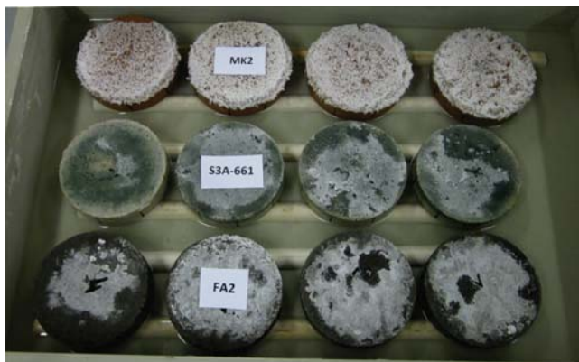
Figure 11.1 Efflorescence of alkali-activated repair mortars based on different precursors (up-metakaolin based mortar, in the middle-slag based mortar, bottom-fly ash based mortar) after water absorption test.
