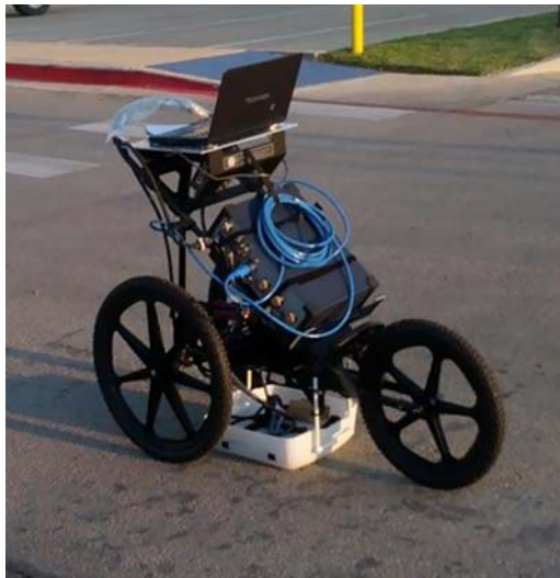
Figure 8.12 Ground penetrating radar equipment.
