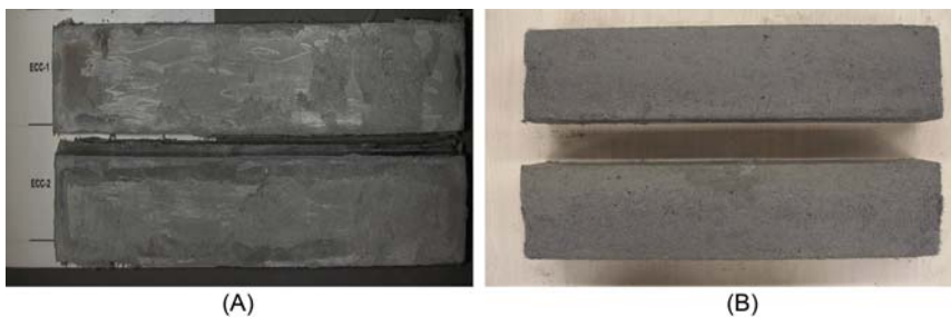
Figure 15.6 Surface appearance of standard Engineered Cementitious Composites (ECC) after (A) de-icing salt surface scaling after 50 F/T cycles (B) after 300 F/T cycles without de-icing salt.
