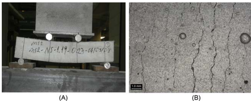
Figure 15.4 (A) Response of Engineered Cementitious Composites (ECC) under flexural loading and (B) typical cracking pattern on positive moment surface of ECC beams.
