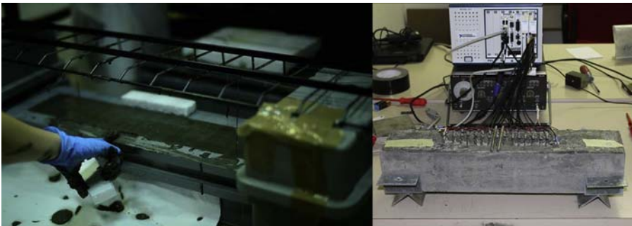
Figure 18.11 SsC in bulk form: casting of a scaled-down reinforced SsC beam (left), wiring of the electrodes to the data acquisition system before testing (right).
