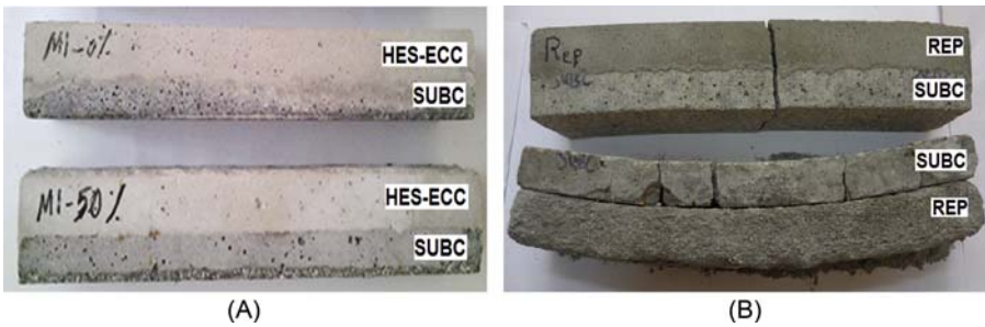
Figure 15.20 Visual observations of layered repair systems (A) high-early-strength–Engineered Cementitious Composites–substrate concrete (HES–ECC–SUBC) system after 300 F/T cycles, (B) repair–substrate concrete (REP–SUBC) system after 150 F/T cycles.
