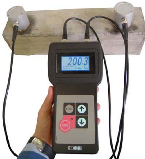
Figure 8.6 Ultrasonic Pulse Velocity test equipment (Controls Group, 2016).
