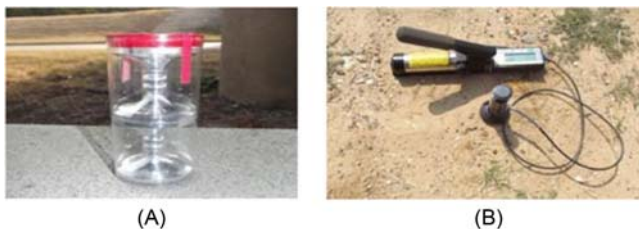
Figure 8.3 ASTM pull-off testing apparatus: (A) testing dollies (B) pull-off adhesion tester (Pallempati et al., 2016).
