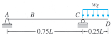
(c) Arrangement of Uniformly Distributed Live Load w_\ell for Maximum Negative M_B
