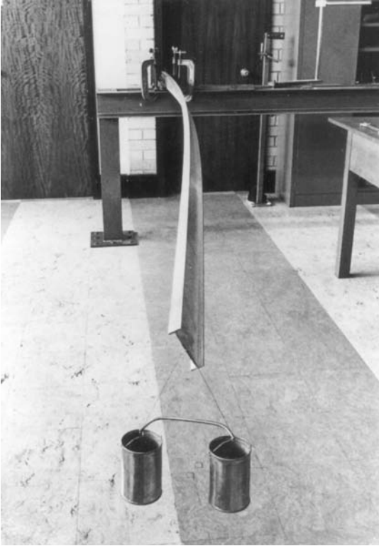
Figure 6.1 Lateral buckling of a cantilever.
