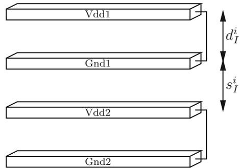
where  $L_{ij}$  is the mutual inductance between the power and ground paths in the two power distribution networks. In general, a power distribution grid with DSDG should be designed such that  $M_{loop}$  is negative with the absolute maximum possible value. Alternatively,
