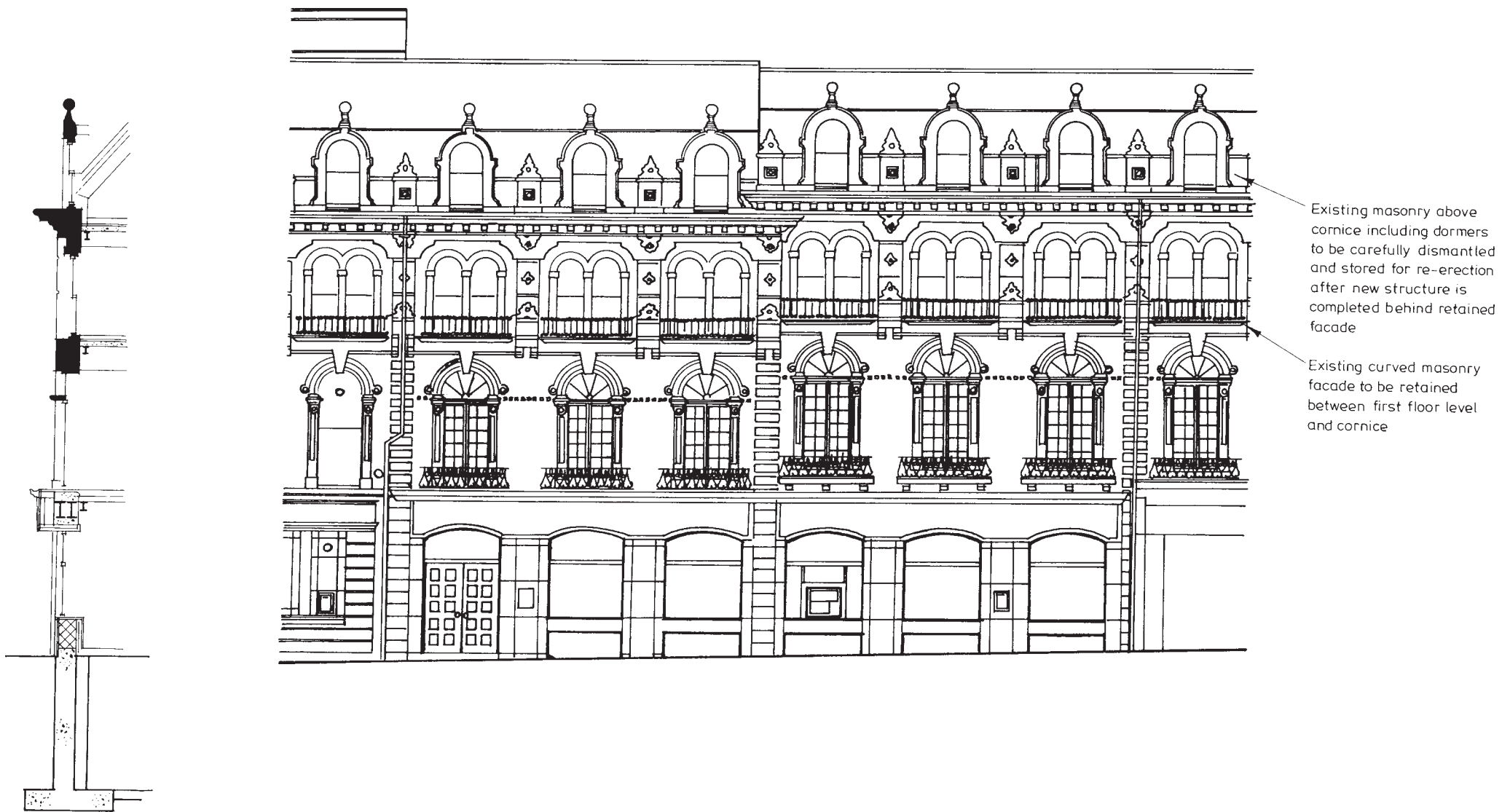
Figure 7.27 Lloyds Bank, Harrogate: front elevation after redevelopment.
