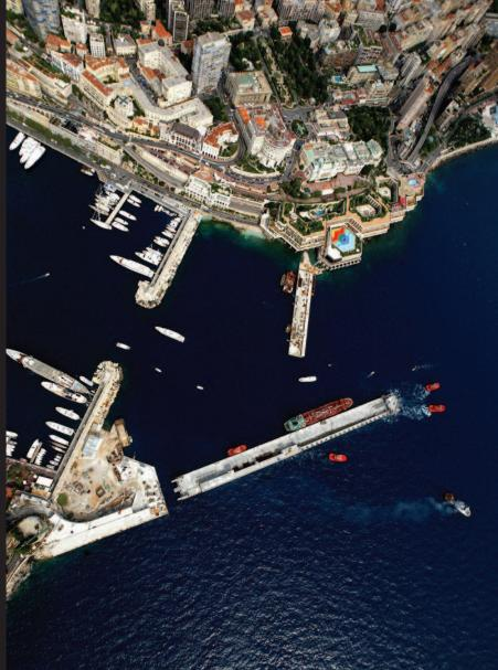
"Breakwaters are normally passive structures designed with only one use in mind. The fact that this project also incorporated a massive car park, a dry dock for recreational craft and extensive retail and administration facilities impressed the Jury as an excellent way of making utilitarian structures useful.
