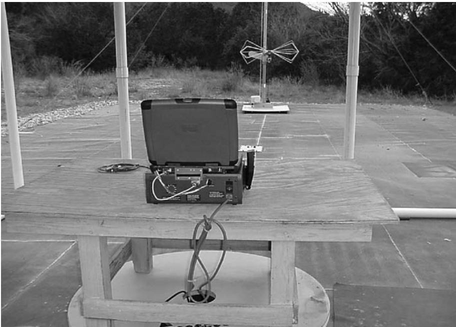
Figure 4.5 A prototype implantable-device programmer is being tested at an open-field test site. The device sits atop a motorized turntable. A biconical antenna is placed 10 m away from the device under test.
