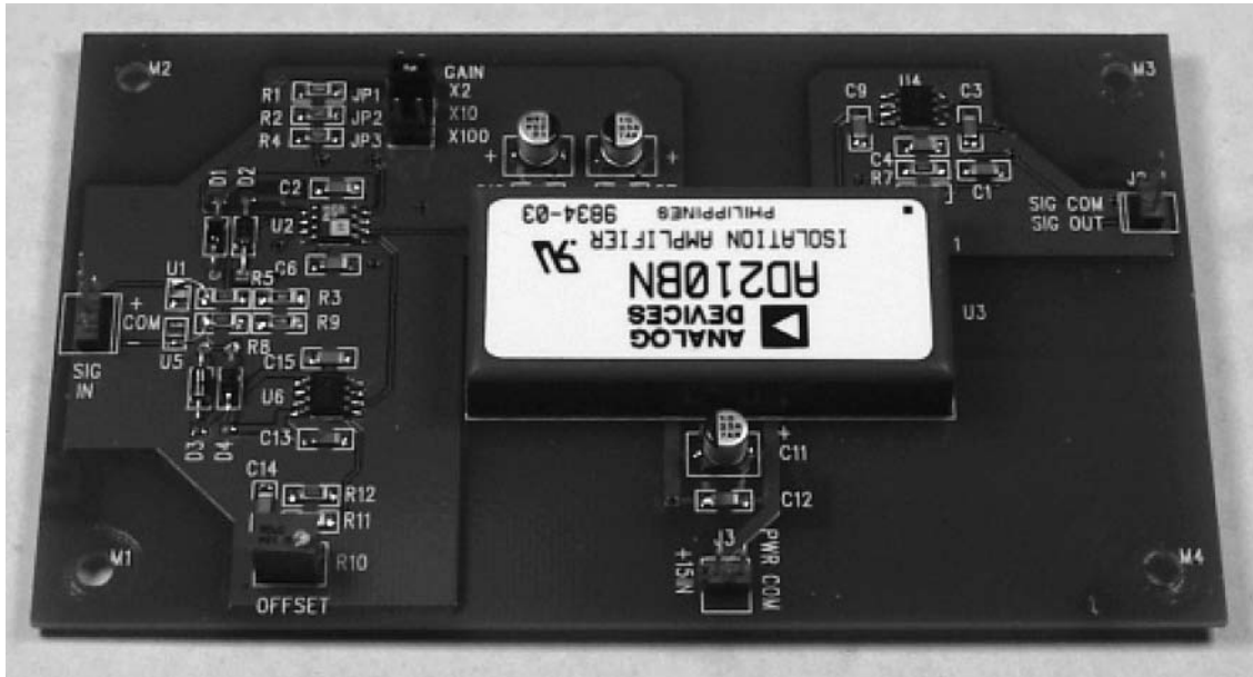
Figure 3.7 This implementation of the general-purpose biopotential amplifier of Figure 3.6 requires a single supply of 15 V at 80 mA, thanks to the AD210's three-port feature.
