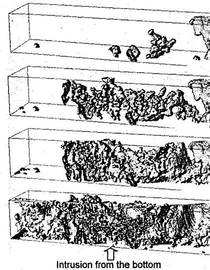
Figure 5. Filling patterns during mercury intrusion from the bottom side for increasing intrusion pressures. We observe first a preferential filling at the right side where the crack is open. With increasing pressure a horizontal fluid flow to the left of the specimen occurs.
