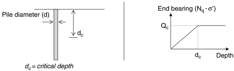
Figure 4.17 Critical depth for end bearing capacity
