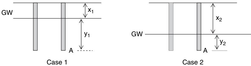
Figure 14.6 Negative skin friction due to groundwater drawdown
