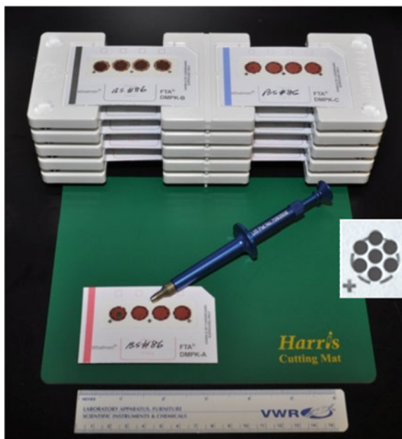
Fig.1 FTA DMPK cards, punch, cutting mat and drying racks from GE Healthcare Corp
