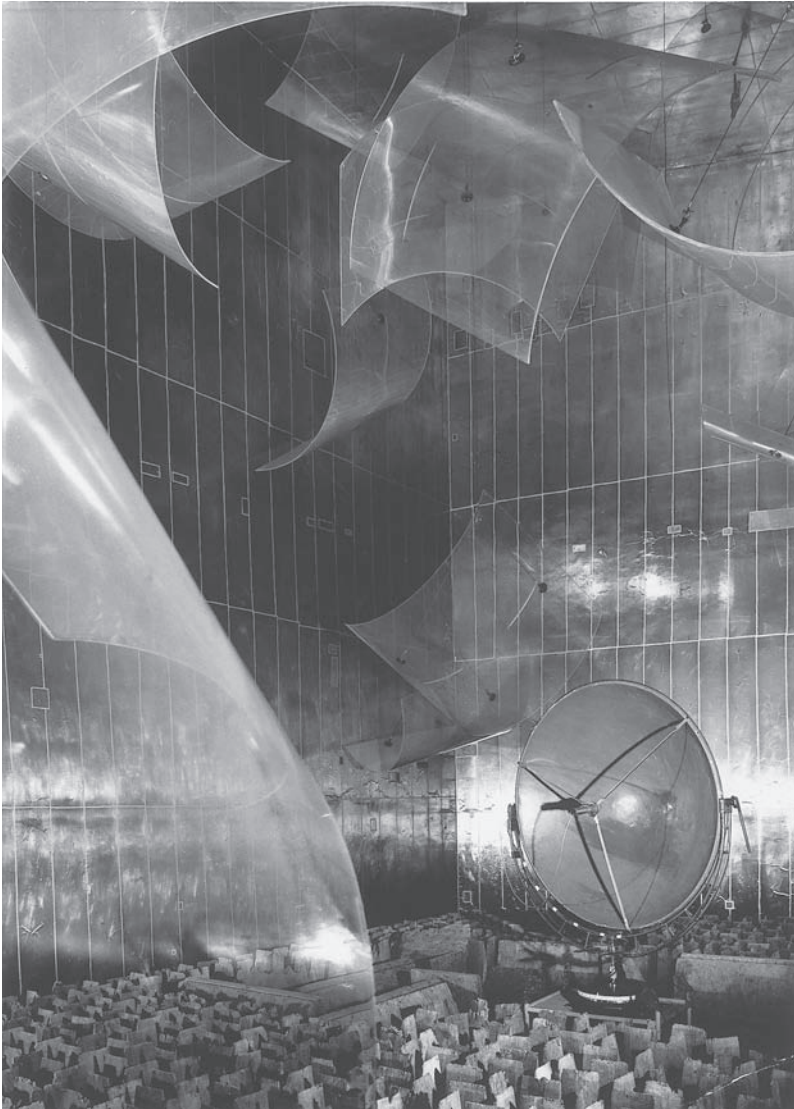
Figure 8.21 Reverberation chamber fitted out with 25 diffusers of Perspex (volume 324 \text{ m}^3 ; dimensions of one shell 1.54 \text{ m} \times 1.28 \text{ m} ).
