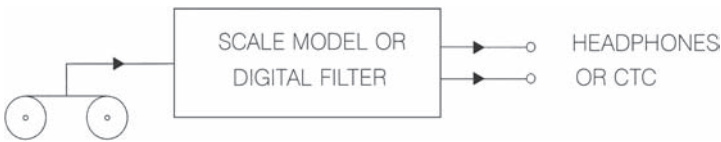
Figure 9.16 Principle of auralisation. The input signal is 'dry' music or speech.
