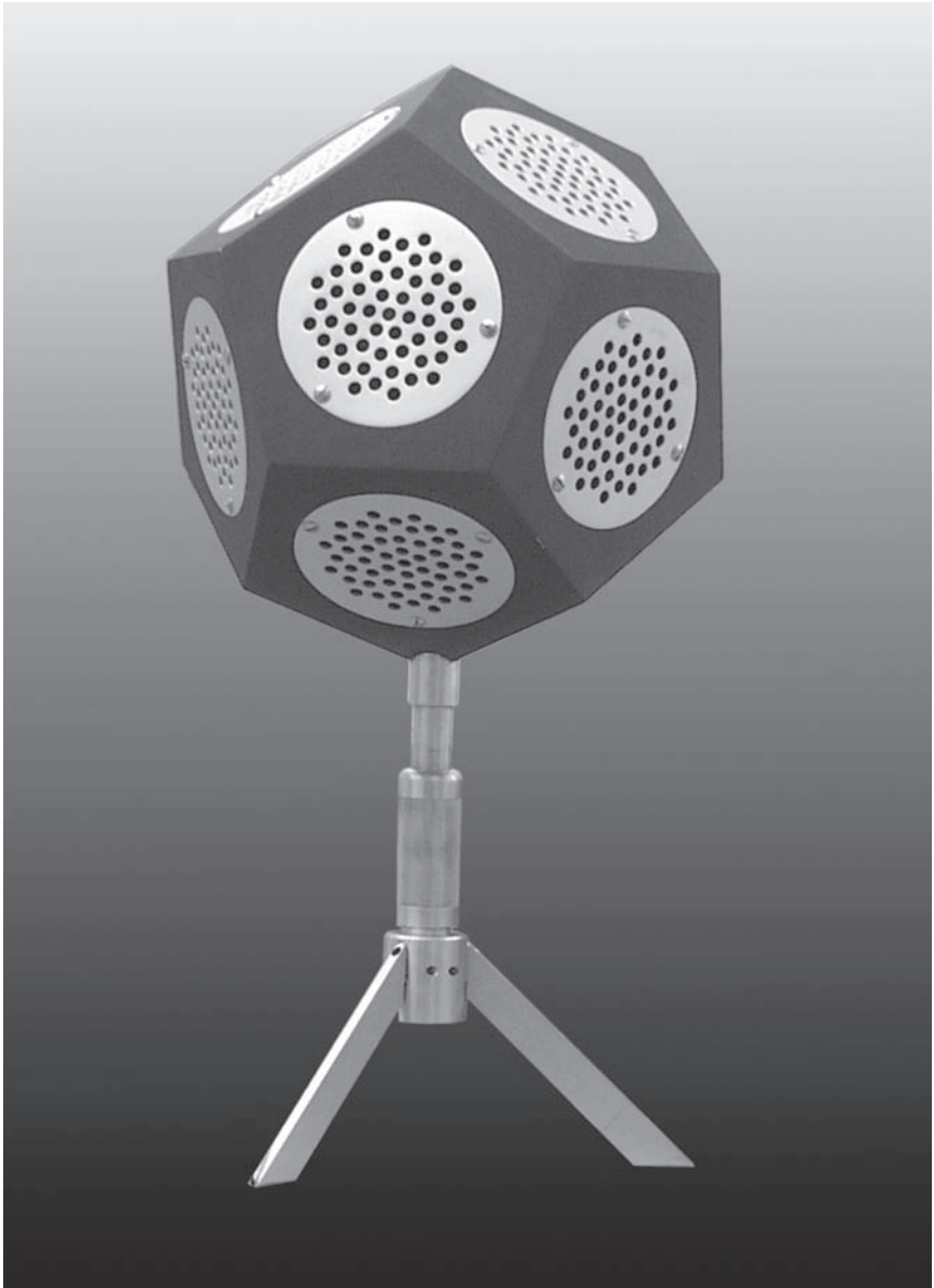
Figure 8.1 Dodecahedron loudspeaker for measurements in room acoustics. (Institute of Technical Acoustics, Aachen)
