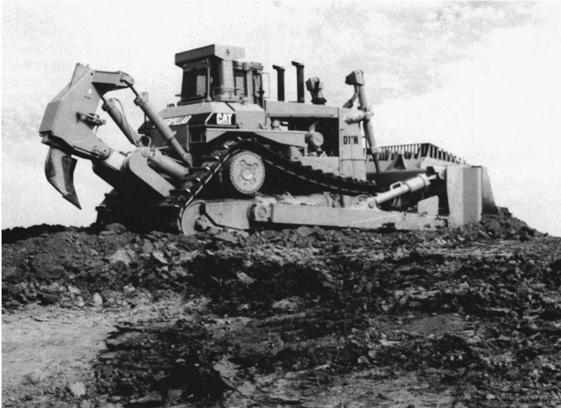
Figure 3-29 D11N Caterpillar Track-Type Tractor with Ripper. Blade Width Up to 20 ft 10 in. (6358 mm), with a Capacity of 42.4 cu yd (32.4 m 3 ). (Reprinted Courtesy of Caterpillar Inc.)
