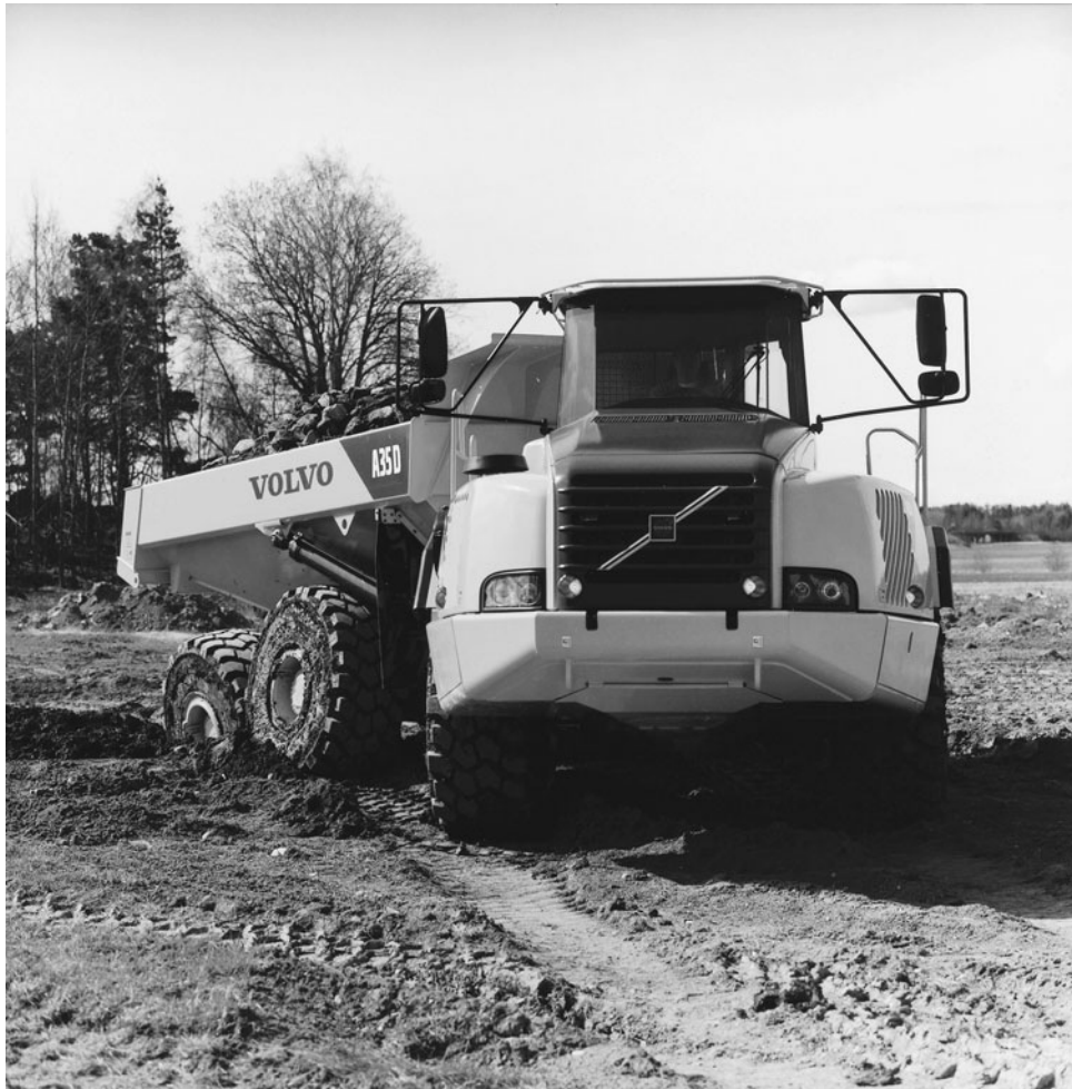
Figure 3-43 Volvo A35D Articulated Hauler. (Reprinted by permission of Volvo Construction Equipment of North America, Inc.)
