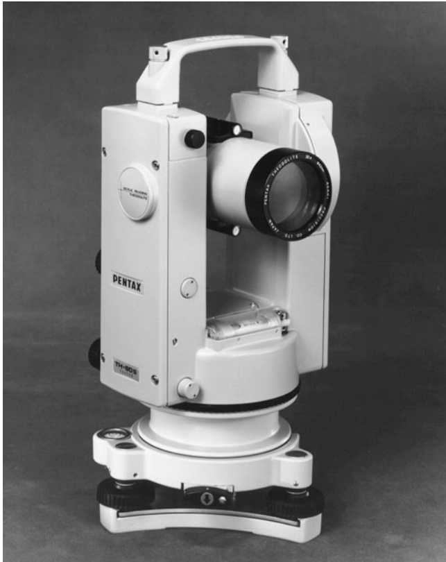
Figure 2-13 Theodolite Available with Internal Lighting System and Optical Plummet. (Reprinted by permission of Pentax Canada Inc.)
