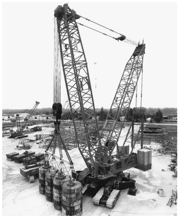
Figure 3-17 Manitowoc Model 21000 Lattice Crawler Crane Has a Base Capacity of 834 U.S. Tons and Can Reach to 640 Feet (195 Metres) with the Luffing Jib Extension Installed. Crawlers of This Size Are Designed Modularly to Allow the Machines to Break Down for Shipping. (Reprinted by permission of Grove Worldwide.)
