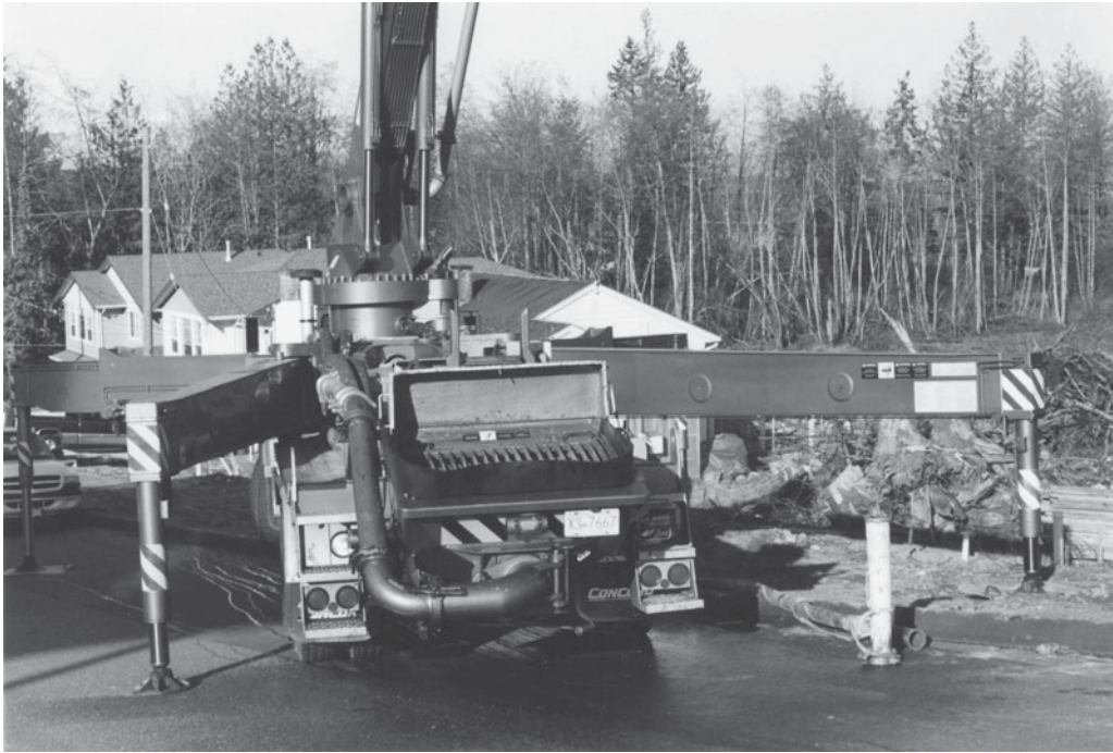
Figure 7-24(a) Truck-Mounted Concrete Pump.
