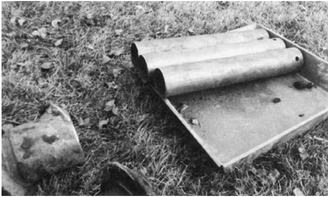
Figure 1-4 Shelby Tubes Used for Obtaining Soil Samples from Test Borehole.
