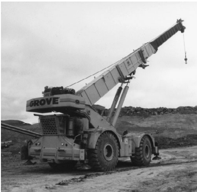
Figure-21 A Pick-and-Carry Rubber-Mounted Crane.
