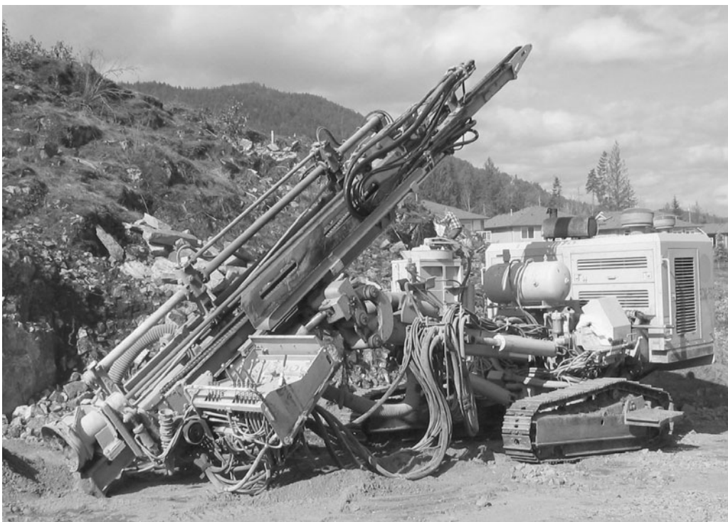
Figure 3-72 Crawler-Mounted Rock Drill Rig.
