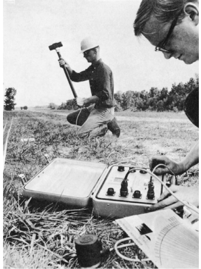
Figure 1-8 Automatic Engineering Seismograph. (Reprinted by permission of ELE International, Soiltest Products Division.)
