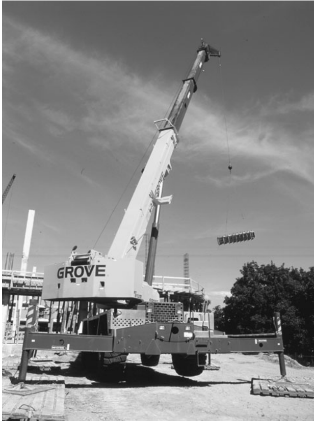
Figure 3-20 Grove RT913E Rough Terrain Crane with a 130 U.S. Ton Capacity. Rough Terrain Cranes Are Used on Unimproved Surfaces. Typically They Have Two Axles and Have to Be Transported to a Job Site. (Reprinted by permission of Grove Worldwide.)
