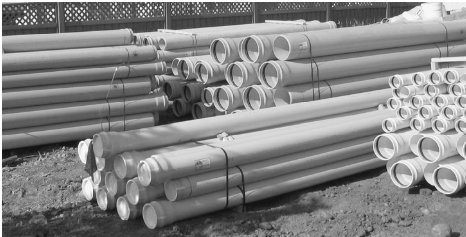
Figure 4-17 (a) Precast Concrete Storm Sewer Pipe Sections. (b) PVC Sewer and Water Pipe.
