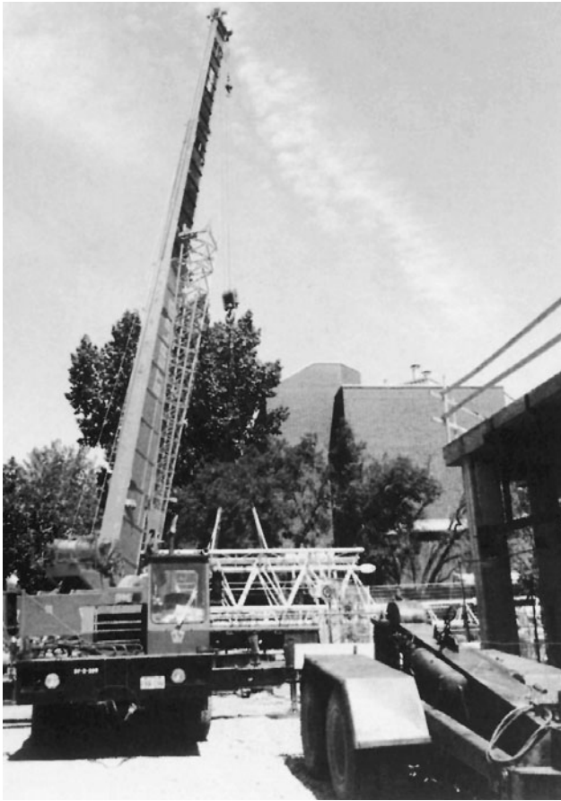
Figure 3-24 Hydraulic Crane with Extended Boom. Note the Jib Being Carried on the Main Section of the Boom.
