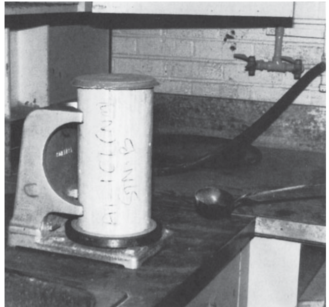
Figure 7-14 Capping Concrete Test Samples.
