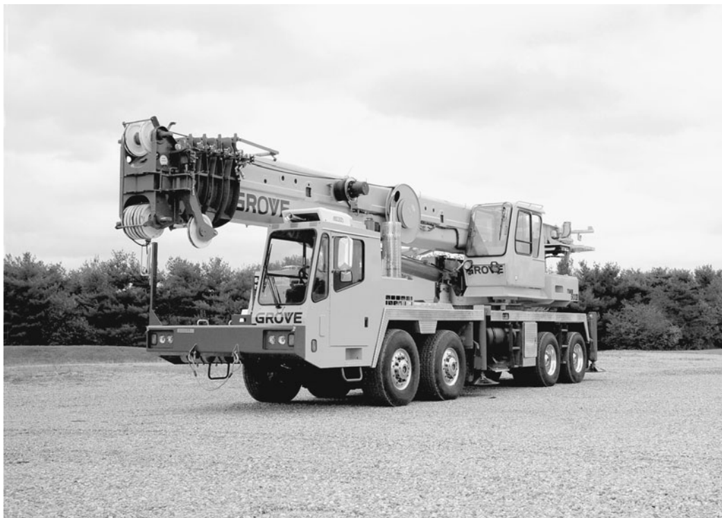
Figure 3-19 The TMS 900E Truck-Mounted Crane Has a 90 U.S. Ton Capacity and with All of Its Inserts and Extensions Installed Can Reach a Maximum Tip Height of 237 Feet (72 Metres). (Reprinted by permission of Grove Worldwide.)
