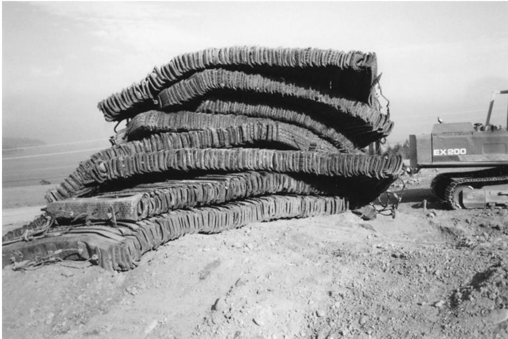
Figure 3-78 Heavy Rubber Blasting Mats.
