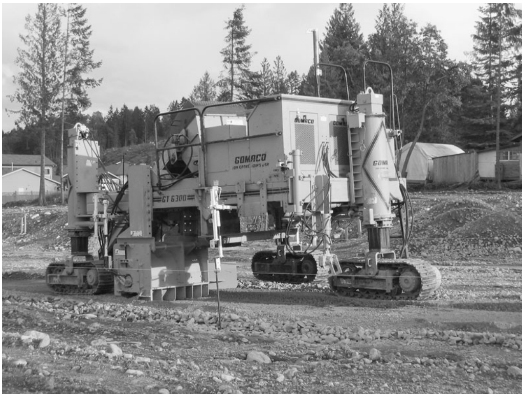
Figure 4-11 Concrete Curb-Forming Machine.
