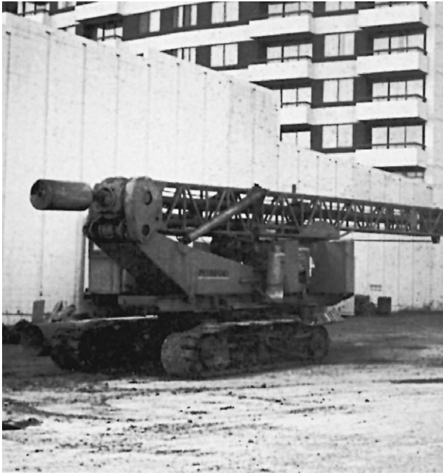
Figure 1-7 Crawler-Mounted Drill Rig.
