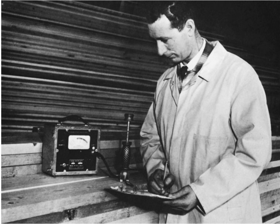
Figure 8-26 Measuring Moisture Content of Laminating Stock with Electric Moisture Meter. (Reprinted by permission of Canadian Wood Council.)
