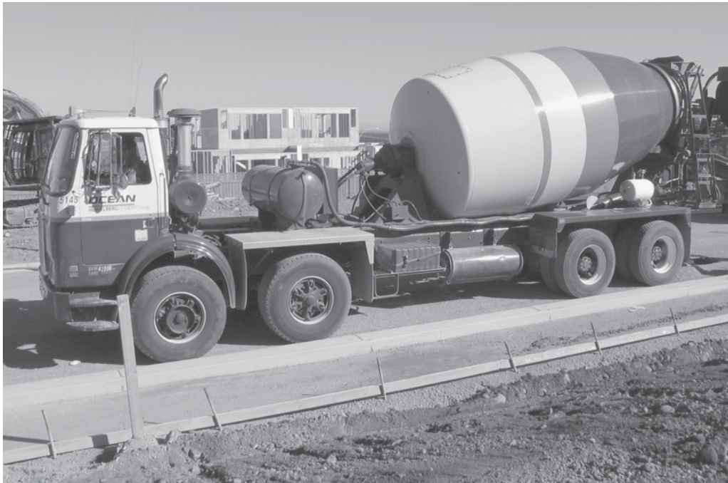
Figure 7-26 Transit Mix Truck.
