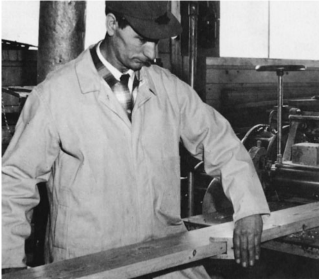
Figure 8-28 Checking Thickness of Laminating Stock with a "Go-No-Go" Gauge as It Comes from Surfacers. (Reprinted by permission of Canadian Wood Council.)
