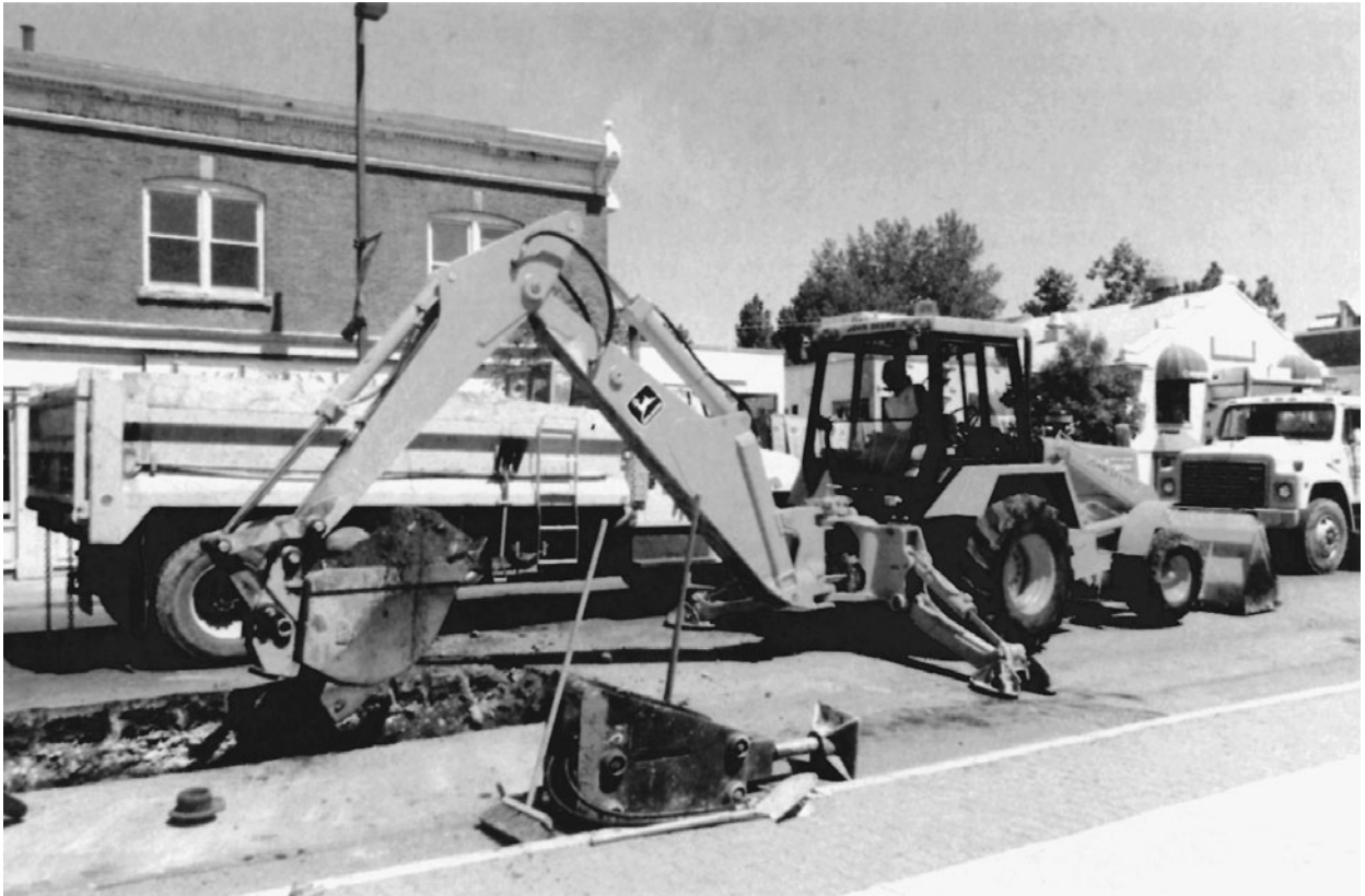
Figure 3-37 Tractor-Mounted Backhoe Equipped with a Front-End Loader. Note the Tamping Attachment on the Ground.
