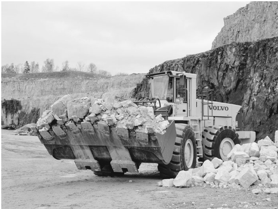
Figure 3-31 Volvo Wheel Loader. Maximum Bucket Size, 18.3 cu yd (14.0 m 3 ). (Reprinted by permission of Volvo Construction Equipment North America, Inc.)
