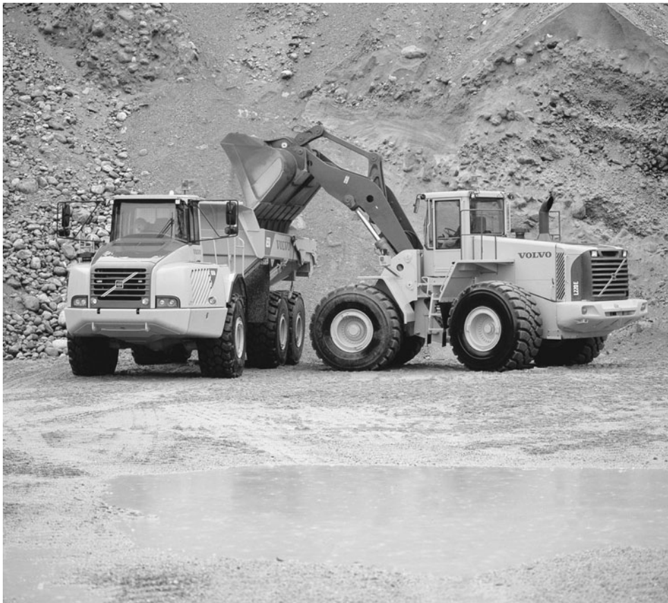
Figure 3-44 Articulated Hauler Being Loaded by a Wheeled Loader. (Reprinted by permission of Volvo Construction Equipment of North America, Inc.)
