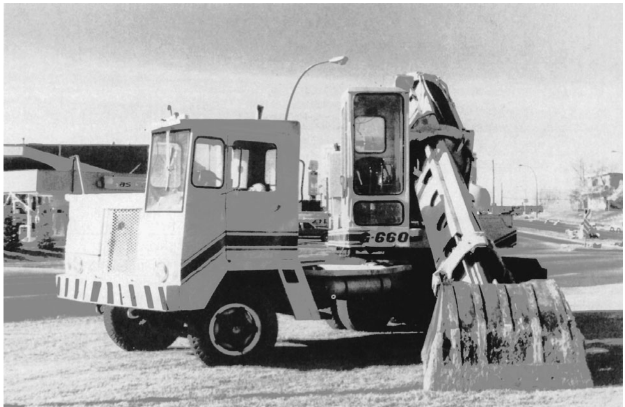
Figure 3-38 Truck-Mounted Excavator with Hydraulic Telescopic Boom.
