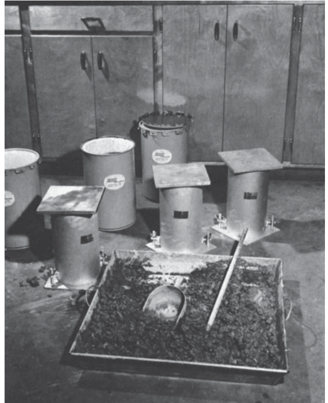
Figure 7-13 Test Cylinders Filled and Covered. (Reprinted by permission of ELE International, Soiltest Products Division.)
