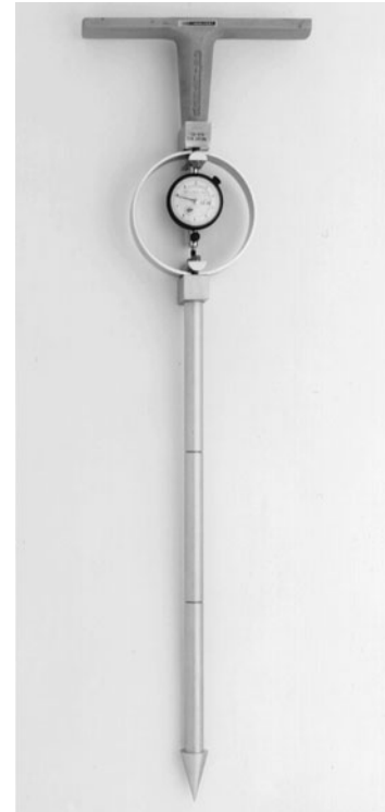
Figure 1-13 Proving Ring Penetrometer. (Reprinted by permission of ELE International, Soiltest Products Division.)
