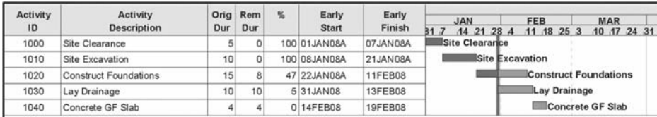
Figure 3.5 Effect of inserting manual progress compared with auto update function.
