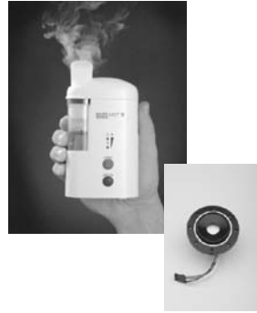
B. Ultrasonic nebulizer with illustrative transducer
