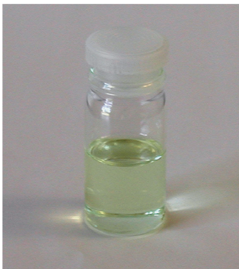
Color Plate 7 AmB nanoparticles from RESOLV in a stable and optically transparent aqueous suspension. (From Pathak et al., 2007a.)
