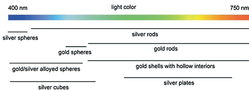
Color Plate 2 A list of silver and gold nanoparticles having various morphologies, compositions and structures, together with their typical locations of surface plasmon resonance bands in the visible regime (Sun & Xia, 2003). (Reprinted with permission from The Royal Society of Chemistry.)
