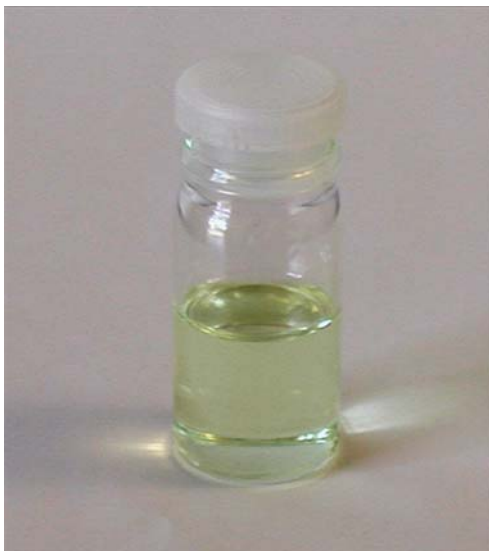
Figure 3.8 AmB nanoparticles from RESOLV in a stable and optically transparent aqueous suspension. (From Pathak et al., 2007a.) (See Color Plate 7)
