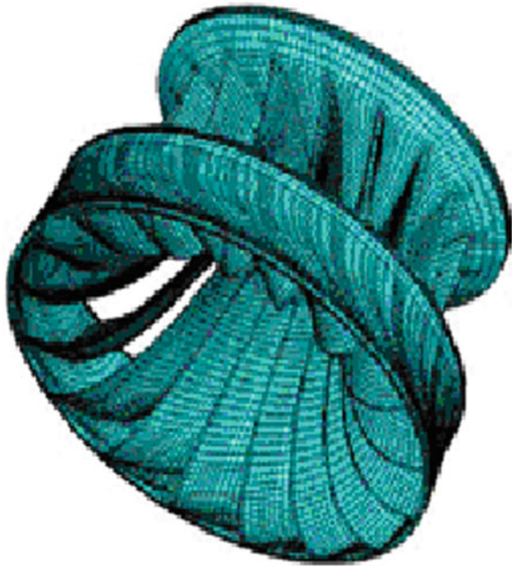
Fig. 1.13 a Runner for three-gorges project. b Blade in machining of runner ( http://www.xsrb.xsnet.cn/xsdaily/gb/content/2005-07/11/content_468089.htm , http://www.slsdge.com.cn )
