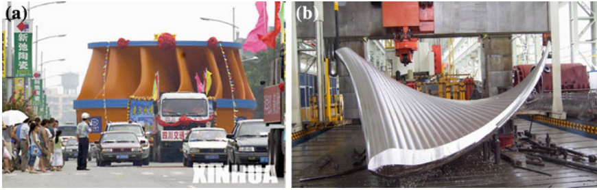
Fig. 1.13 a Runner for three-gorges project. b Blade in machining of runner ( http://www.xsrb.xsnet.cn/xsdaily/gb/content/2005-07/11/content_468089.htm , http://www.slsdge.com.cn )
