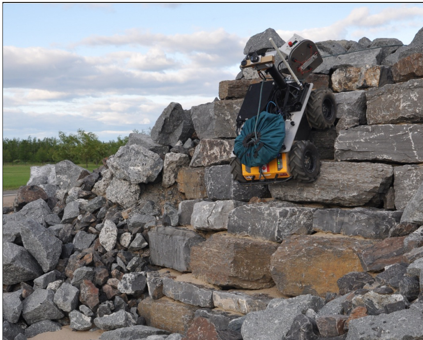
Fig. 1 The vScout prototype operating in steep, rough terrain in the Mars Emulation Terrain at the Canadian Space Agency in St. Hubert, Quebec, Canada, June 2013. Video from this test is available at: http://youtu.be/z5ud7k9ozvQ
