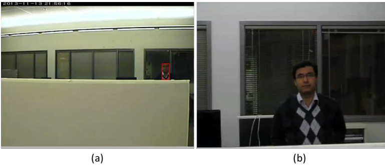
Fig. 5 Result of another indoor experiment (a) shows position of the detected moving object by stationary camera, and (b) shows position and close-up of the moving object in moving camera after PTU motion
