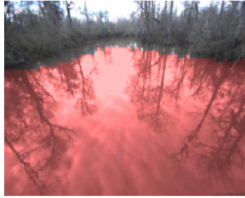
Fig. 2 Pixels with probability greater than .5 after river segmentation are classified as river and marked red [1]. They are then projected onto river plane to create an initial map of the environment. This image is from a dataset taken from McCarthy river, Mississippi.
