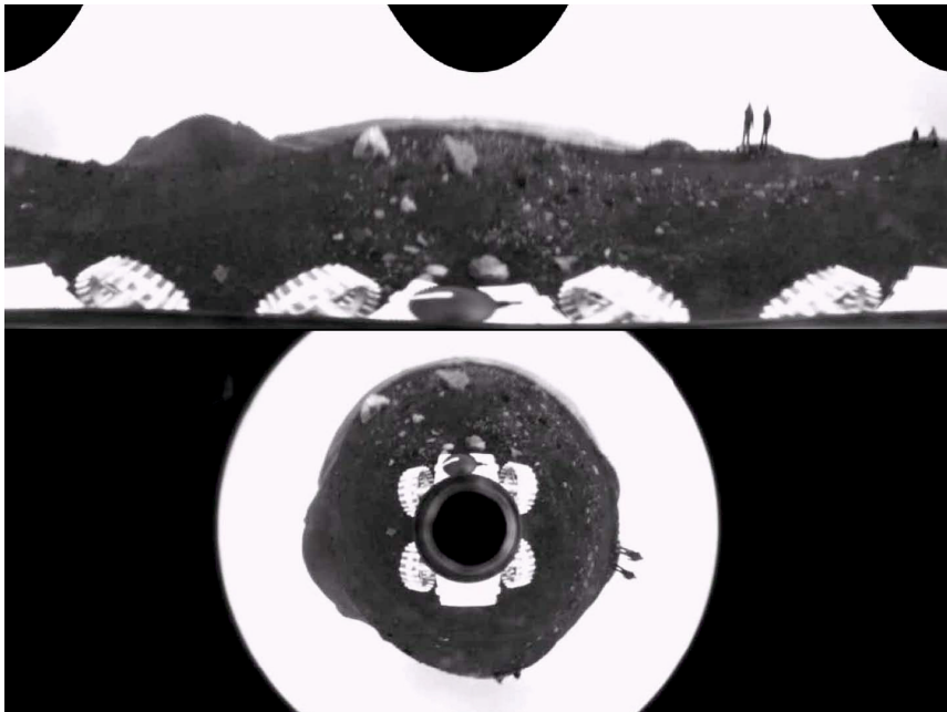
Fig. 4 Omnicamera raw image (bottom) and corresponding panoramic projection (top)
