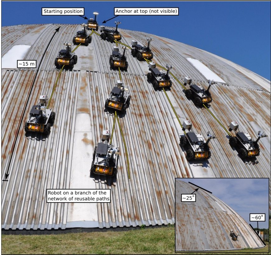
Fig. 9 A time-lapse view of the vScout operating on the Dome at UTIAS. The vScout used a network of reusable paths. It was manually taught a path and then it was able to autonomously repeat that path to return to any previously visited point.
