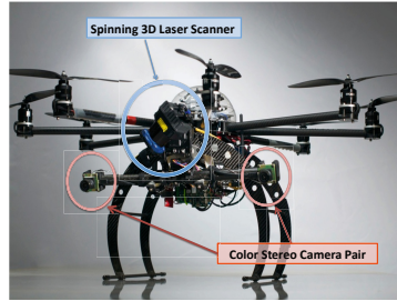
(c) Vehicle local sensing consists of a lightweight spinning laser scanner and stereo color camera pair.
