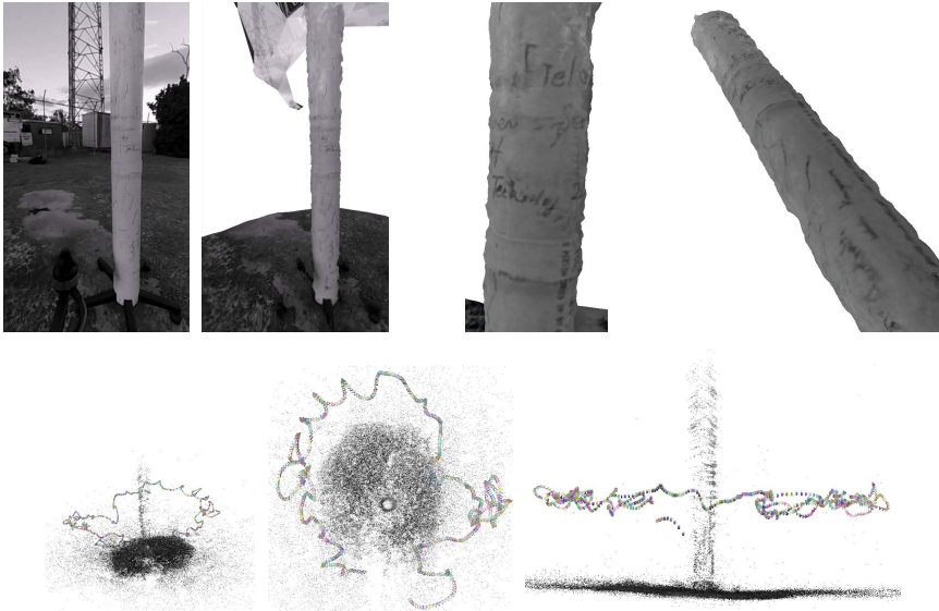
Fig. 14 3D pole reconstruction results. An original image (top left) and various views of the texture-mapped surface (top row). SfM-based camera trajectory estimation (bottom row). The scale of the trajectory is arbitrary, up-to-scale, since we use a monocular camera.
