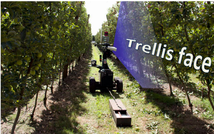
Fig. 1 Apple Orchard, Warburon 3799, Victoria. The research ground vehicle Shrimp traversing between two trellis rows, scanning one side using a LiDAR.
