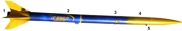
Fig. 3 Final rocket: 1) gimballed nozzle, 2) parachute bay, 3) camera, 4) IMU, motor and payload section, 5) antenna
