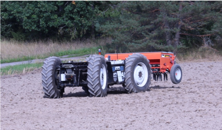
Fig. 1 APU-Module, the autonomous tractor
