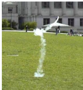
Fig. 1 In the absence of aerodynamic forces, a bare solid rocket engine spins out of control. A stabilizing controller is therefore necessary on a minirocket LV
