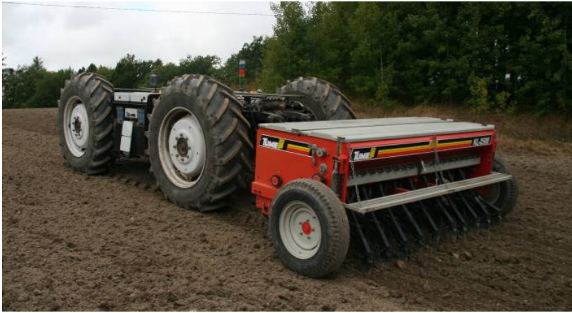
Fig. 2 APU-Module with the seed drill, Tume KL-2500 in the field trial
