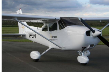
Fig. 8 The data-gathering aircraft, fitted with a Novatel SPAN INS/GPS Navigation system and downward facing camera for site detection
