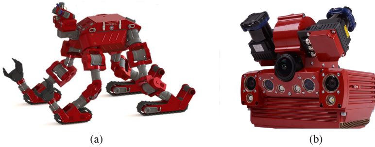
Fig. 1 A rendering of CHIMP in four limb driving mode (a). CHIMP's tracks and joints are fitted with encoders for odometry. Its torso contains a Honeywell Inc. HG9900 IMU. Close-up of CHIMP's head (b), containing Pixim Inc. Seawolf cameras in a stereo configuration for visual odometry along with other perception sensors.
