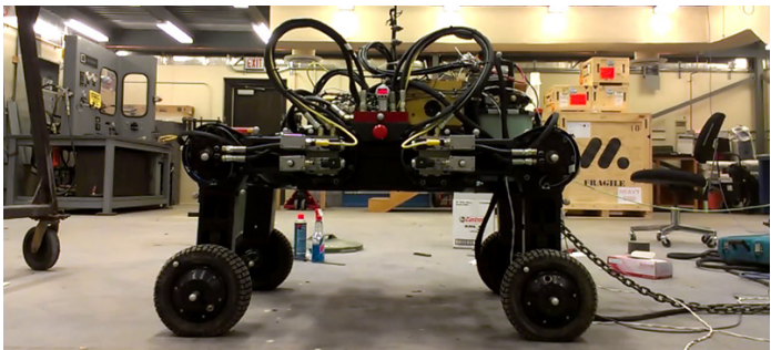
Fig. 2 MHT in home configuration , where all hip and knee joints of all legs are set to 0^\circ
