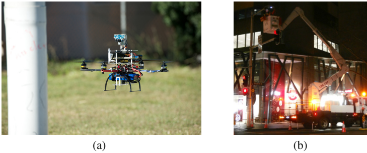
Fig. 1 (a) Our MikroKopter platform hovering relative to a pole in the foreground. (b) Traditional pole inspections can require lengthy setups and road blockages for vehicle access which disrupts traffic.
