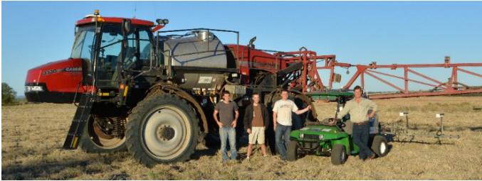
Fig. 1 The small robot platform (green) shown next to a typical farm spray machine (red) with humans for scale. While the robot shown here is a research platform it is approximately the size envisaged by the work in this paper.
