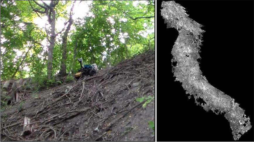
Fig. 10 The vScout in the ravine (left). A 3D model of the terrain from the first test using VT&R on the ravine wall (right). The model was made using Mobile Scene Modeler (mSM) from MDA.
