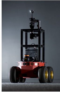
Fig. 5 An ActivMedia P3-AT robot equipped with an omnidirectional vision system.
