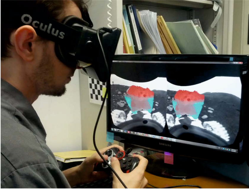
Fig. 7 Mission specialist's graphical interface, with a rendered view of fused camera and LRF data for each eye. A joystick is used to control the mobility system.
