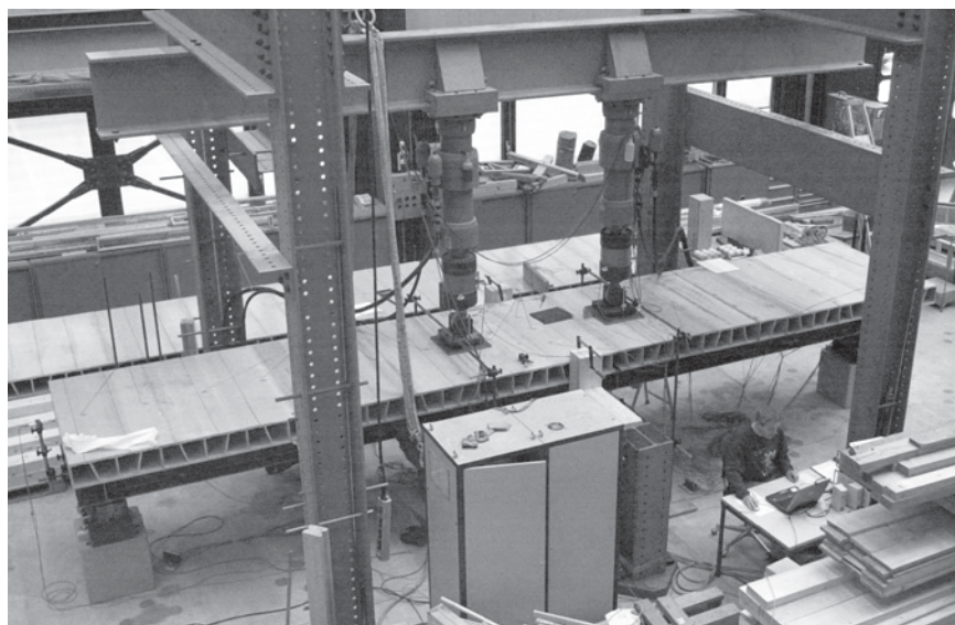
12.14 Set-up of hybrid FRP-steel bridge girders with adhesive connections (longitudinal set-up).
