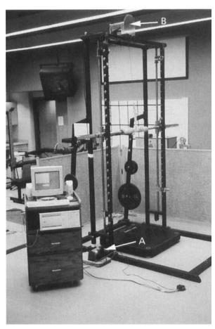
Fig. 3.5 The Ballistic System is an example of the application of the latest technology to strength training. A computer constantly monitors movement of the barbell using a linear transducer (A) providing feedback of force, velocity and power during the athlete's performance. An electronic brake (B) can be used to limit the impact forces and eccentric load on the athlete or to modify the concentric resistance profile.
