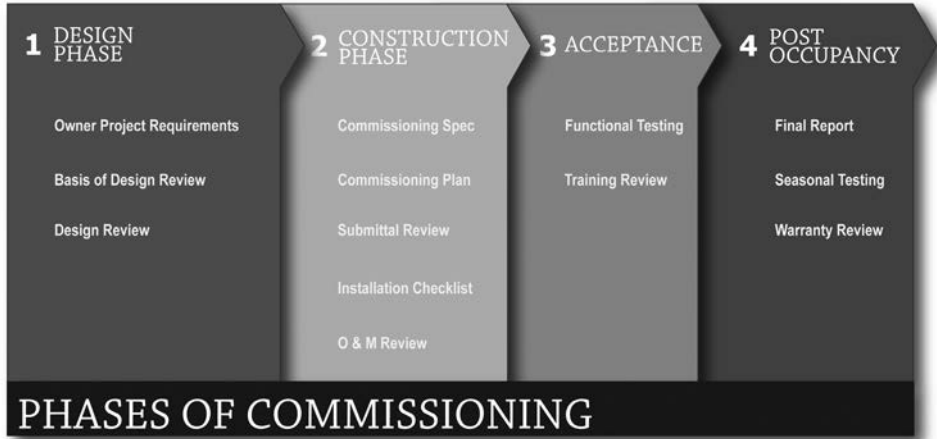
FIGURE 13.1 Phases of commissioning.
