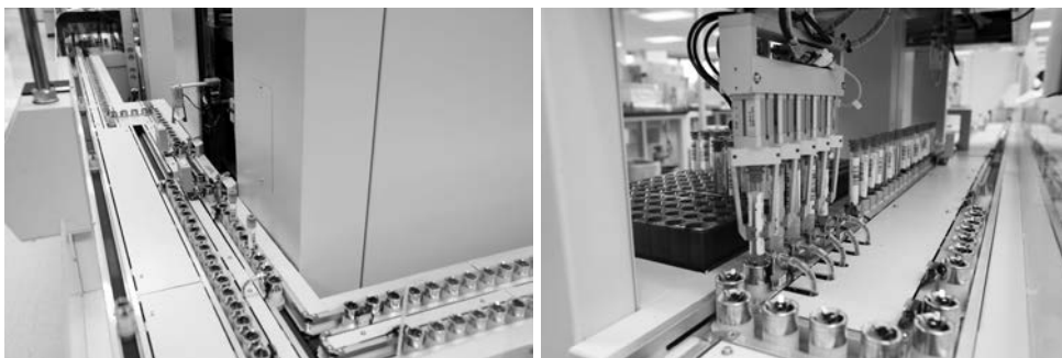
FIGURE 11.16 Laboratory track system. (Courtesy of Beckman Coulter, Inc.)
