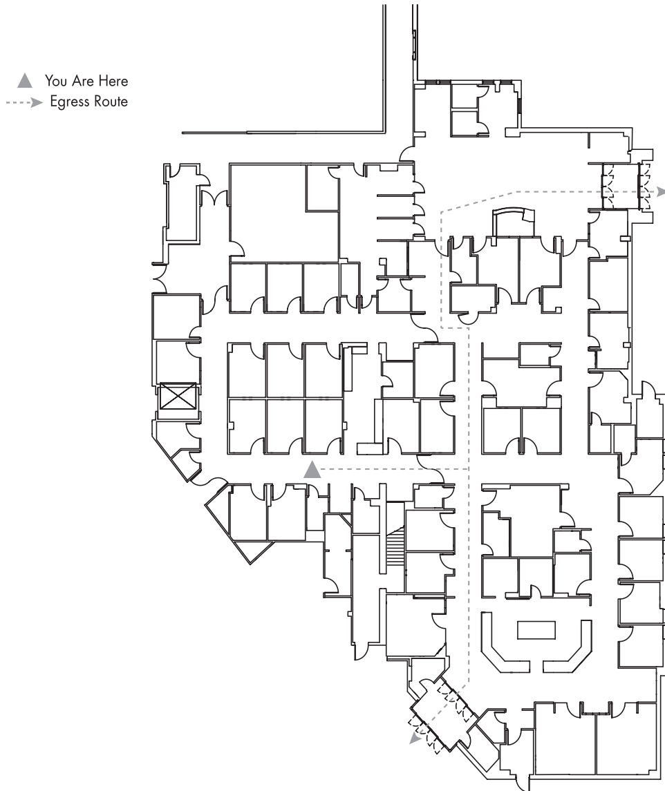
FIGURE 2.5 Emergency exit or life safety plan. (Courtesy of Thomas, Miller & Partners, Brentwood, TN.)
