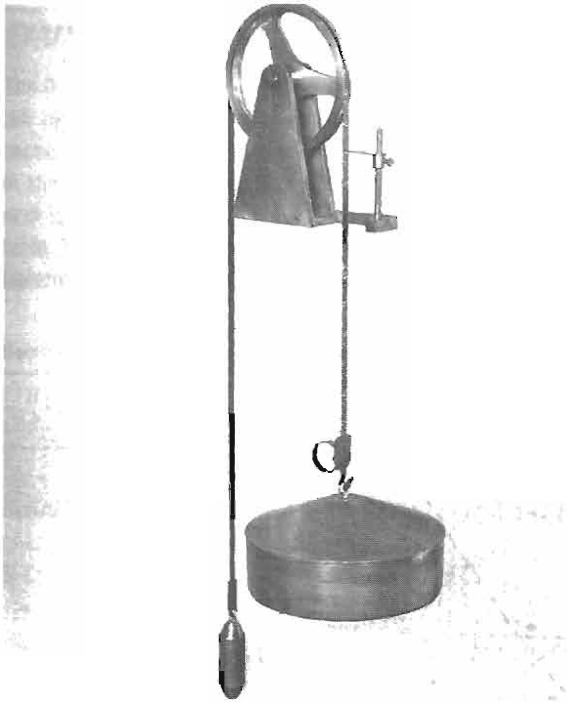
FIGURE F-11 Simple float-counterweight system for measuring water-surface elevation. The pulley can be attached to a recorder to obtain a continuous record. From Buchanan and Somers (1968).
