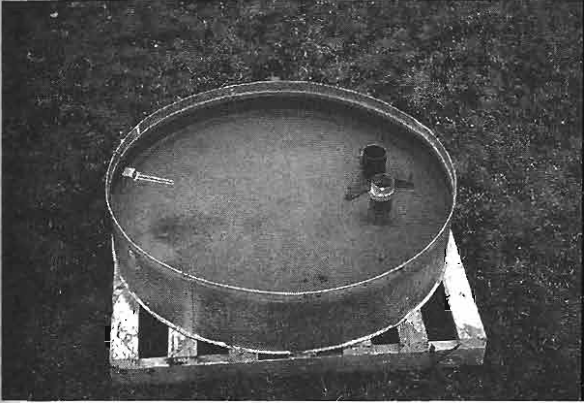
FIGURE 7-5 Standard U.S. National Weather Service “Class-A” evaporation pan. The pan is 4 ft (1.22 m) in diameter by 10 in. (25.4 cm) high and set on a low platform. The stilling well in which water level is measured is on the right, and a floating thermometer is on the left. Typically an anemometer is installed next to the pan and a rain gage must be located nearby. Photo by author.
