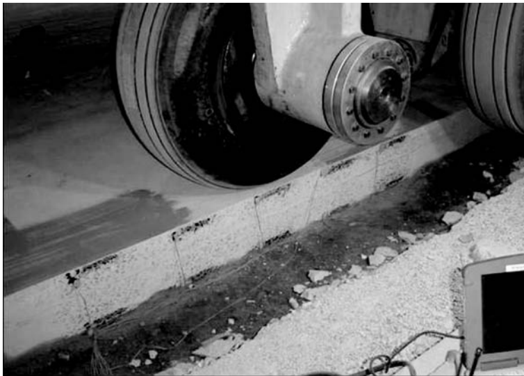
(b) The 13.2 ton (30,000 lbs) singlewheel load was above gages 5 and 6
