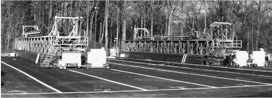
Figure 1. The FHWA two ALF machines loading pavements at PTF site.
