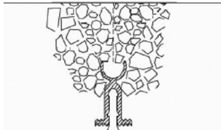
Figure 13. Vertical crack where the bar was placed.
