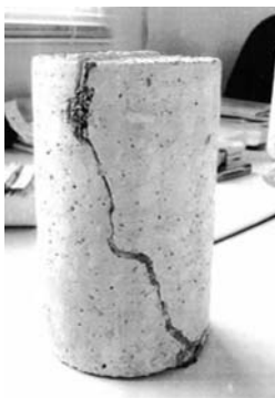
Figure 2. Core with induced crack by the JRI+ system.
