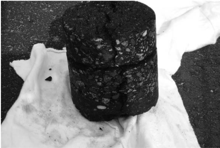
Figure 7. Premature reflective cracking between MP 0.2 and 2.5.
