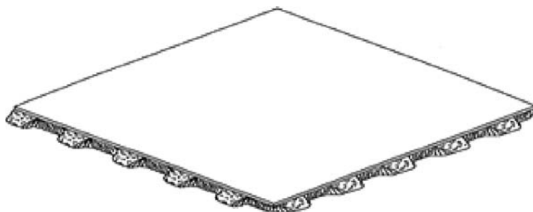
Figure 1. Resulting slab with interlocking hinged boundaries.
