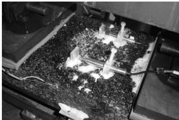
Figure 3. Soapy water is currently used to detect the appearance of cracks (Somda 2007).
