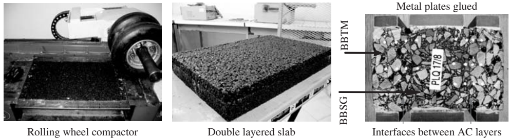
Figure 3. Preparation of the slab and the sample in laboratory, and photograph of obtained sample.
