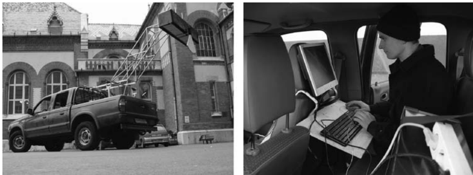
Figure 2. The instrument platform mounted on the pickup and the controlling environment.
