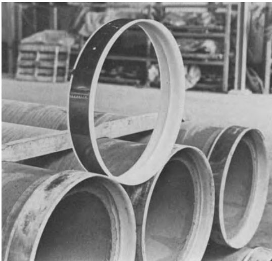
Fig. 115. Polyvinyl chloride-steel sleeves, attached to polyurethane beaded plain-end pipes to effect a compression joint
