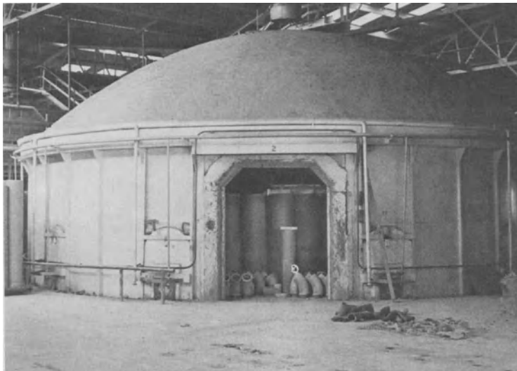
Fig. 87. Round downdraft kiln used in the sewer pipe industry
