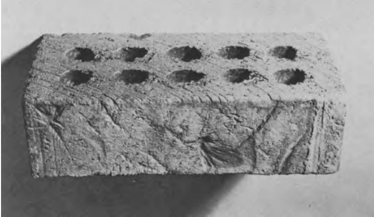
Fig. 104. Face-brick texture with a natural motif applied by a roller
