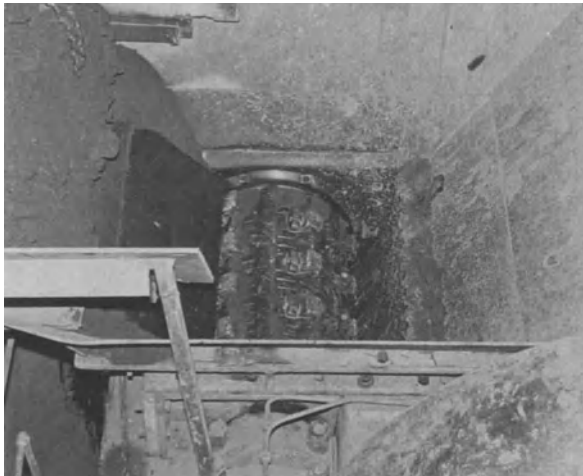
Fig. 23. Single-roll crusher receiving a charge of shale as mined
