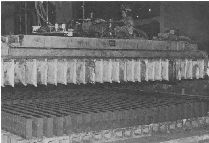
Fig. 54. Automatic setting of stiff-mud face bricks on a kiln car deck
