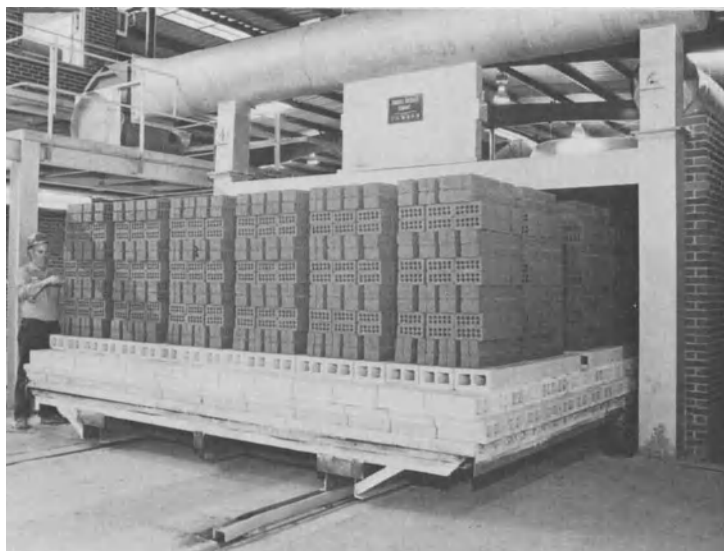
Fig. 86. Kiln car emerging from a wide tunnel kiln. Courtesy of Swindell-Dressler Co.
