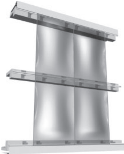
22.27. (above) Cross-stiffening studies for the façade of the VAKKO Headquarters building in Istanbul, Turkey (expected completion in 2008), designed by REX (Joshua Prince- Ramus and Erez Ella).
