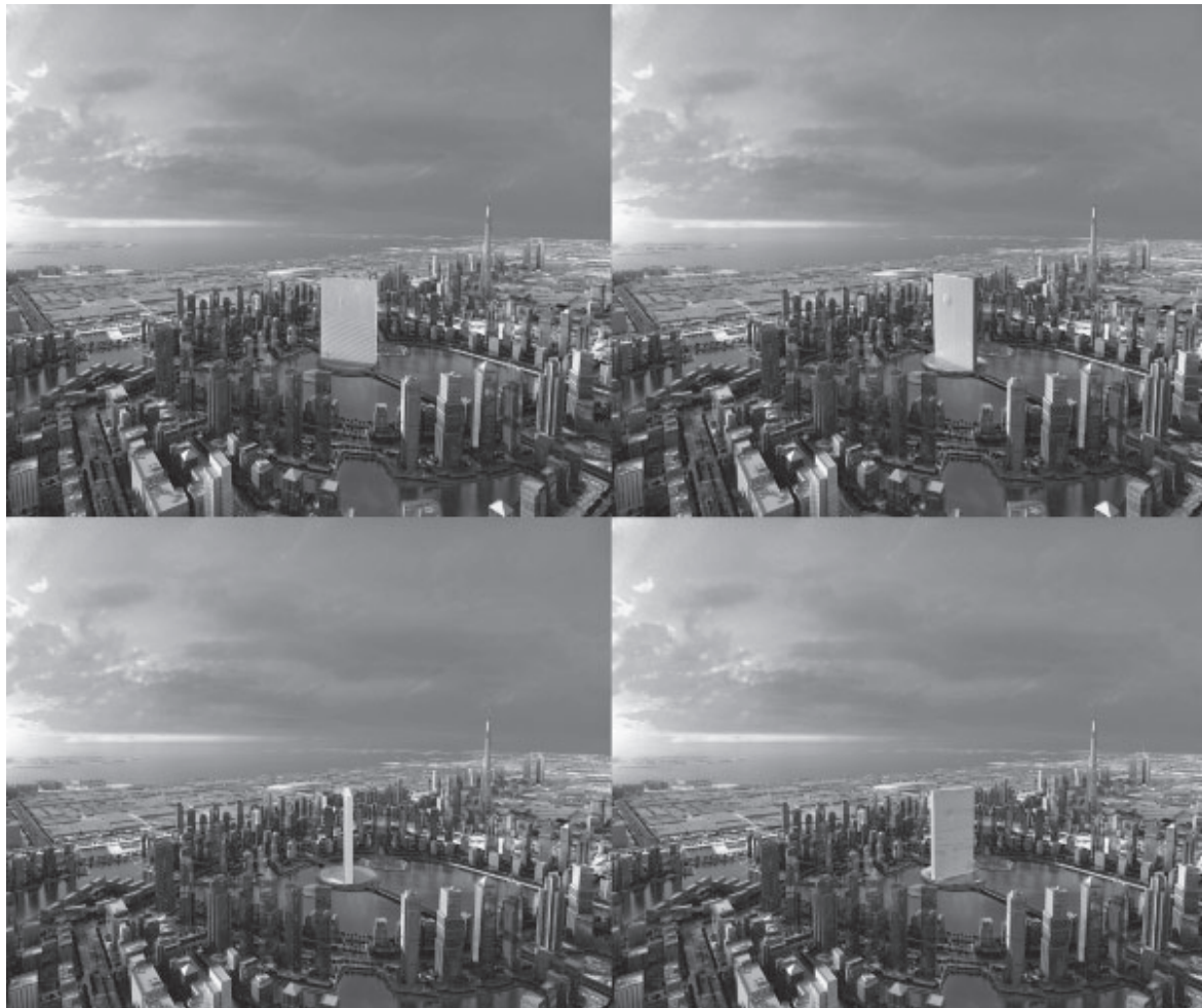
21.5a–d. The Dubai building would rotate around its vertical axis, so that main façades would receive no direct sunlight.
