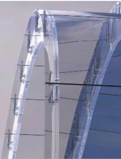
22.5. (right) SCL Glass Showroom : a rule-based, associative parametric model was developed in CATIA.
