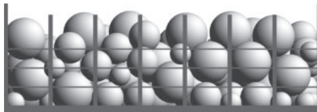
9.16a–b. (below) Gantenbein Vinery: elevation images of the digital "basket" were used to create the "grape- like" brick wall patterns.
