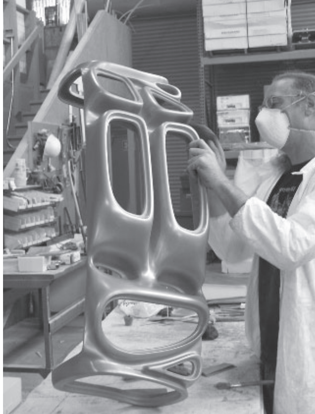
19.19. UniBodies : sculptor Scott Van Note hand finishes the surface of a metallic fiberglass composite.
