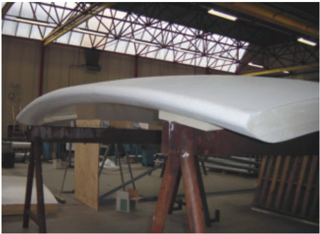
20.16. Yitzhak Rabin Center: the prototype of the composite sandwich shell for the roof wings.
