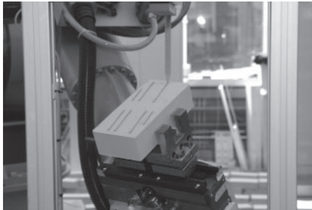
9.21. Gantenbein Vinery : the robot also applied the bonding agent to the bricks.
