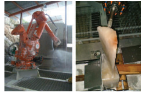
22.46. Baha'i Mother Temple : the alabaster panels would be milled with a 5-axis CNC milling machine.
