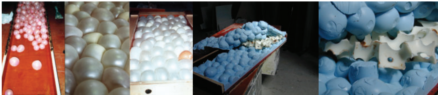
21.17a–e. Sponge : one of the test studies consisted of casting resin in the mold filled with silicon-covered, water-filled balloons.
