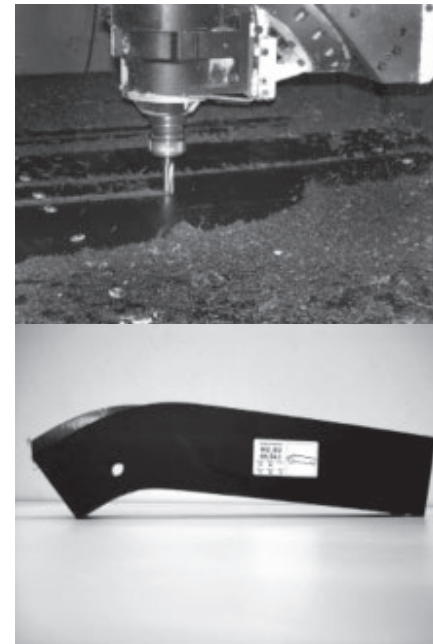
18.12a. Hungerburg Funicular Stations : CNC-cutting.
