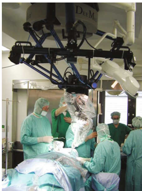
Fig. 1.8 The SurgiScope, a Delta robot carrying a 70 kg microscope (courtesy of ISIS)
