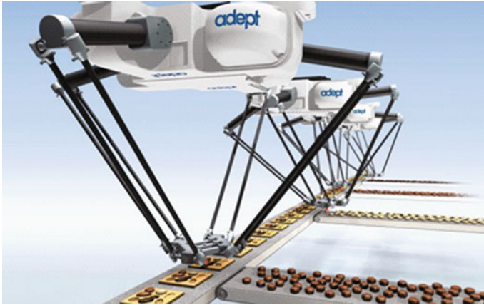
Fig. 1.4 Adept Quattro robots picking and placing chocolates (courtesy of Adept)
