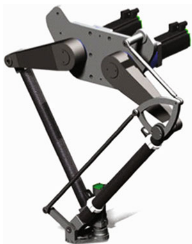
Fig. 1.14 Examples of robots with 2 DOF able to position a device with constant orientation in a plane: Robot PacDrive Delta 2 (courtesy of Schneider Electric)
